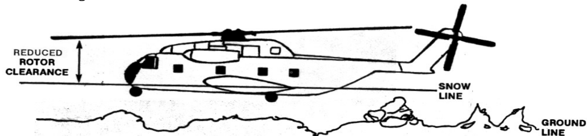
Figure 4005-1: Increased Rotor Hazard / Potential Obstacles Below Snow Surface
