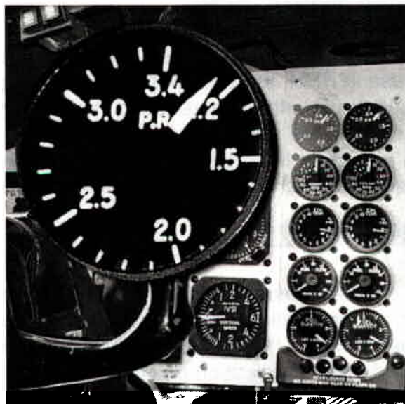
Figure 3.1-15 Pressure Indication Gauges
