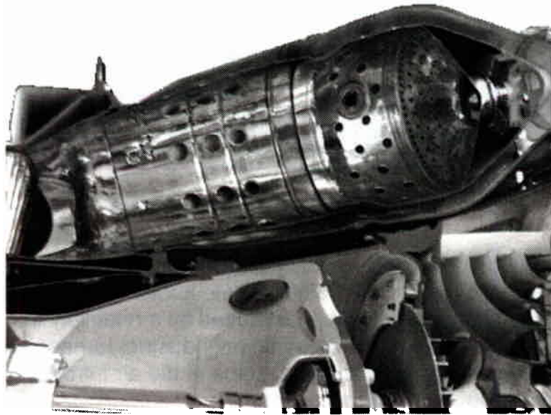
Figure 3.2-16 Can Type Combustion Chamber
