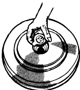
1 Removing Arming Plug From Mine.
