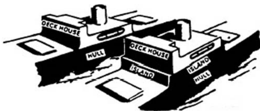
Figure 30 – Differences between deckhouse and island.
