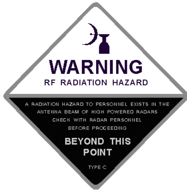
Figure 4-17.—Sample of one type of radhaz sign.
