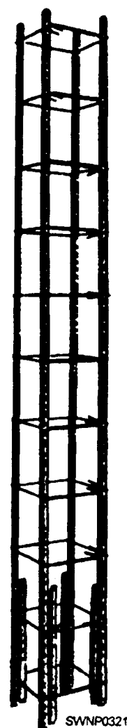
Figure 7-9.—Column steel in place.
