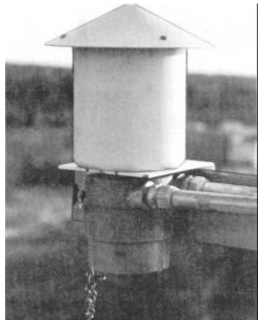
Figure 2-11.—ML-643/GMQ-29 dew-point sensor.
