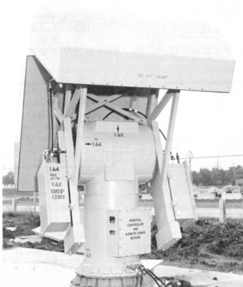
Figure 1-25.—AN/SMQ-11 dual frequency array antenna.
