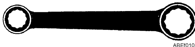
Figure 1-30.—12-point box-end wrench.
