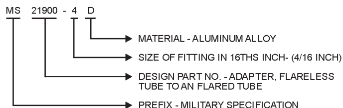
Figure 10-25.—Typical styles of MS fittings.
