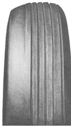
Figure 7-28.—Rapid tread wear caused by misalignment.
