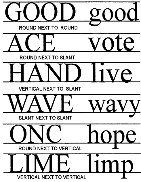
Figure 5-38. —Common spacing problems.
