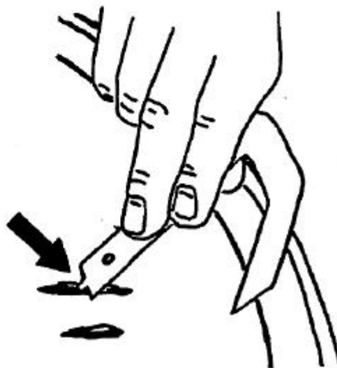
Figure A-5. Gauging defective wheels.
