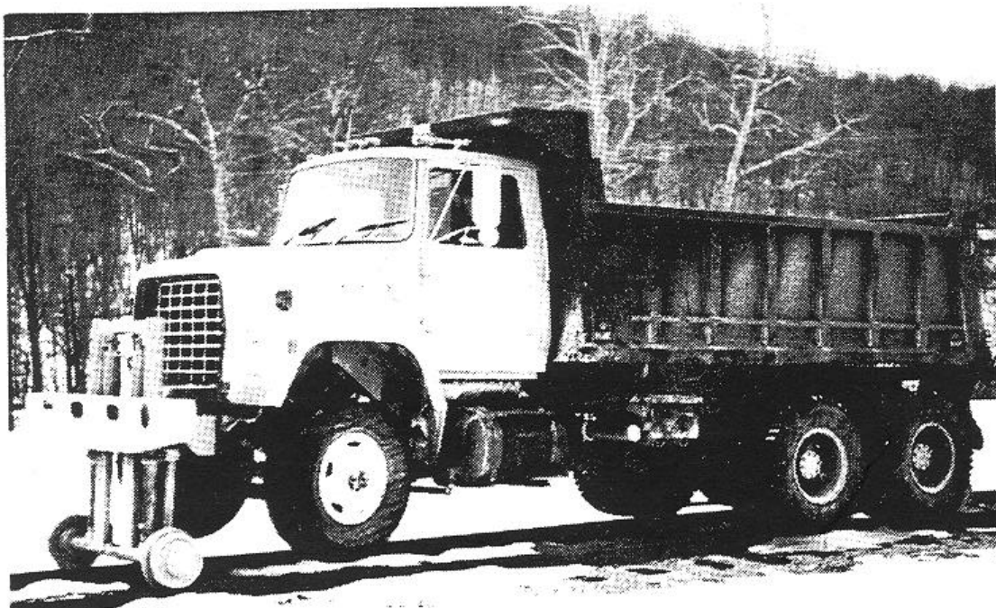
Figure 2-18. Example of a hy-rail vehicle.
