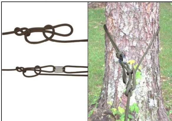
Figure 10-21. TRANSPORT TIGHTENING SYSTEM
