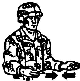
Figure 071-326-0608-29. Move in Reverse (for Stationary Vehicles)
