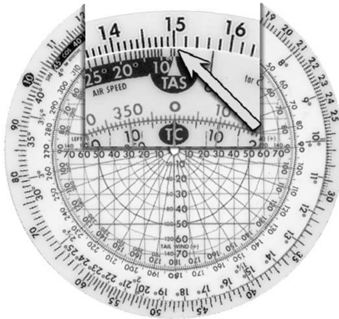
Figure 4.6-5 In-Flight Wind Calculation 1
