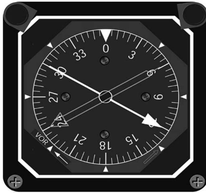
Figure 4.1-3 Remote Gyro Vertical Compass Card
