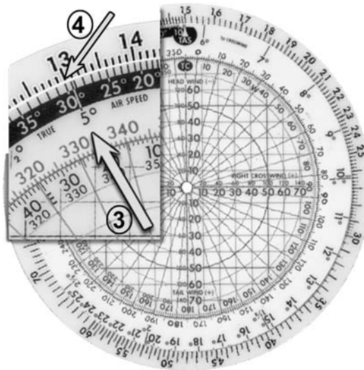
Figure 4.6-7 In-Flight Wind Calculation 3 & 4
