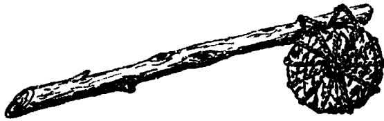
Figure 2-42. Typical pole charge.
