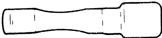
Figure 4-7. Chinese Communist stick-type defensive hand grenade.
