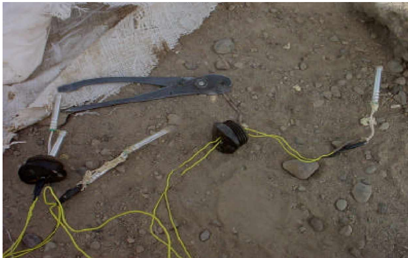
Plastic shipping caps for former Soviet Union 122mm Projectiles modified to accept a blasting cap
