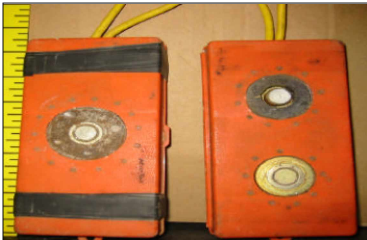
Improvised Explosive Device plastic boxes with detonating cord and stereo speaker magnets, to affix on metal target.
