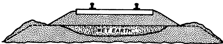
Figure 4-32. Effect of a water pocket under the middle of ties.
