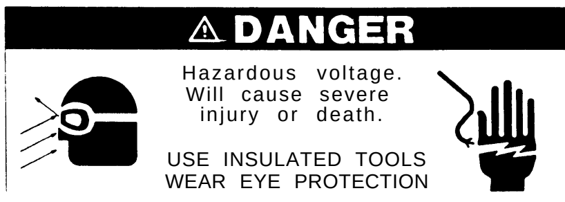
Figure 14-1. Battery warning sign
