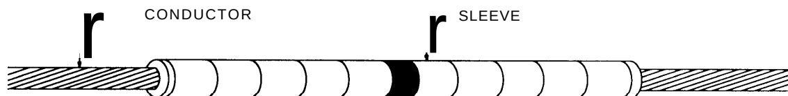
Figure 4-12. Single-sleeve compression splice (Courtesy of BURNDY Electrical)
