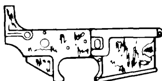
CORRODED WITH HOLE (NONREPARABLE)
