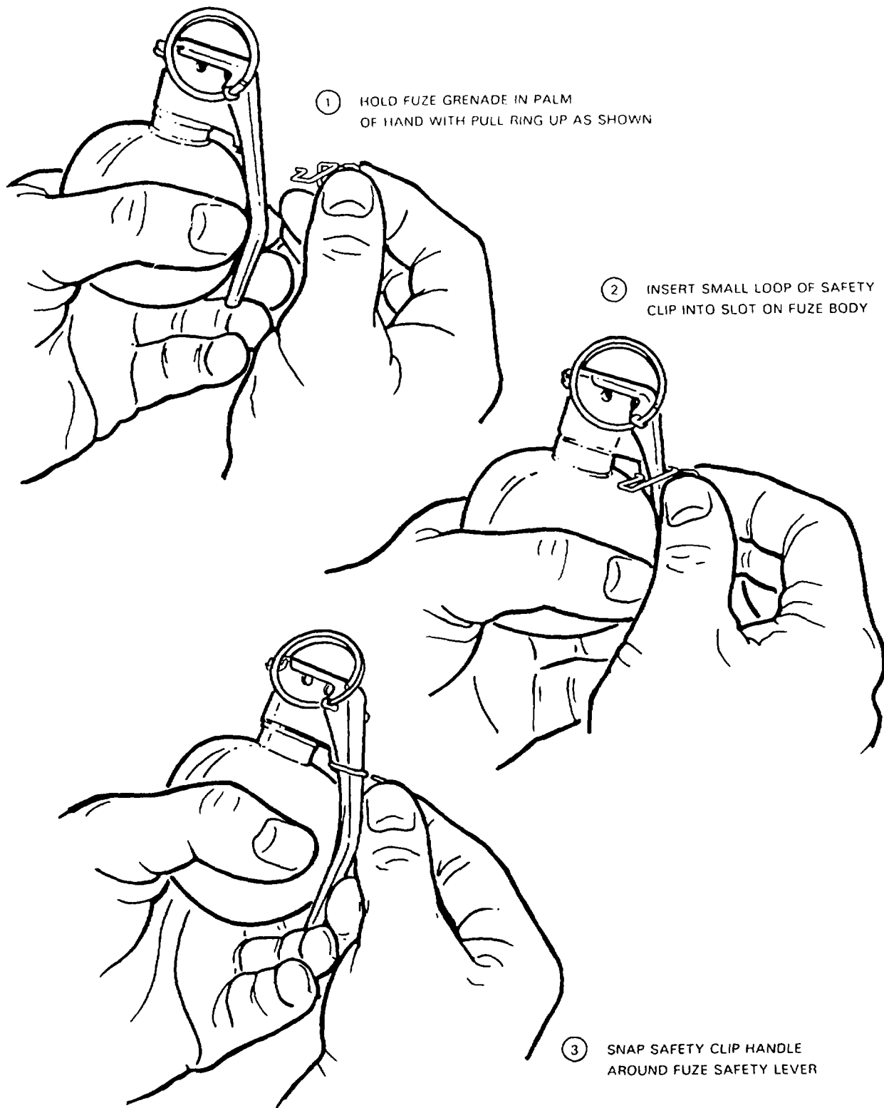
Figure 3-5. Assembly of safety clip to grenade M67.
