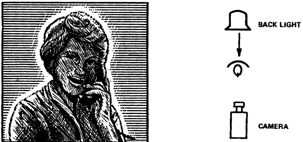
Figure 4-7. Rimming or halo effect by using back lighting
