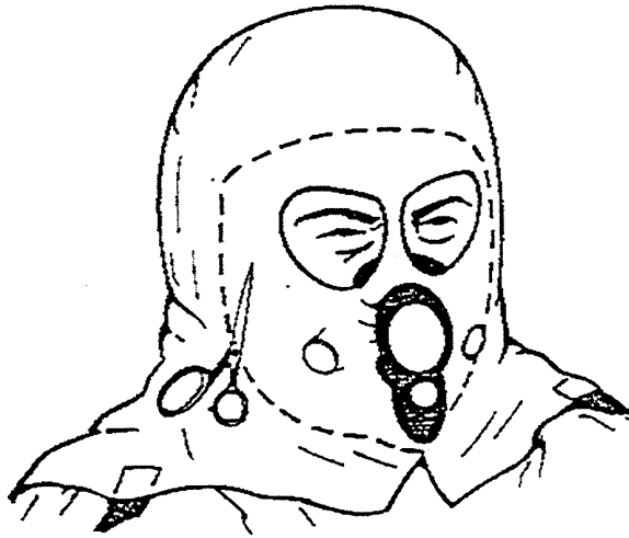
Figure 3-1. Cutting off the hood.
