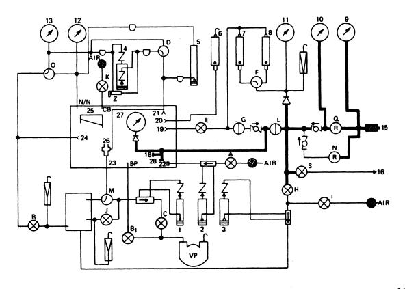
Figure 2-4.—Model 1172AS100 regulated high pressure N<sub>2</sub>system.
