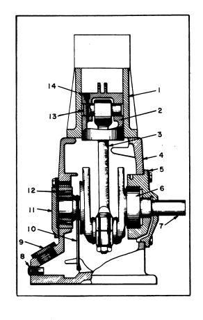
1. Crosshead guide8. Drain plug2. Crosshead9. Oil filler cap3. Connecting rod10. Oil ring4. Crankcase11. End plate5. End plate12. Roller bearing6. Roller bearing13. Wrist pin7. Crankshaft14. Retaining pin
