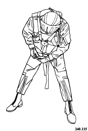
Figure 5-7.—Aircrewman attaching leg straps.
