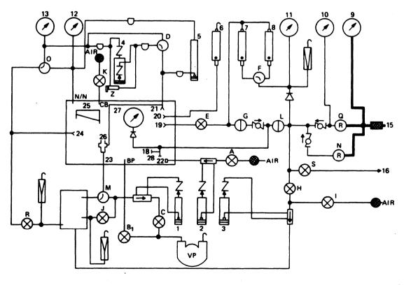
Figure 2-3.—Model 1172AS100 supply nitrogen system.
