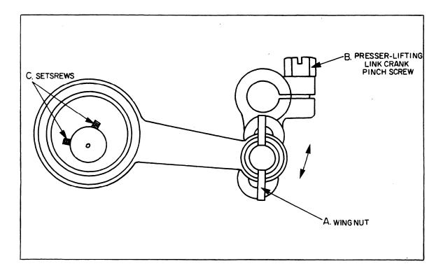
Figure 4-10B.—Presser-lifting eccentric.
