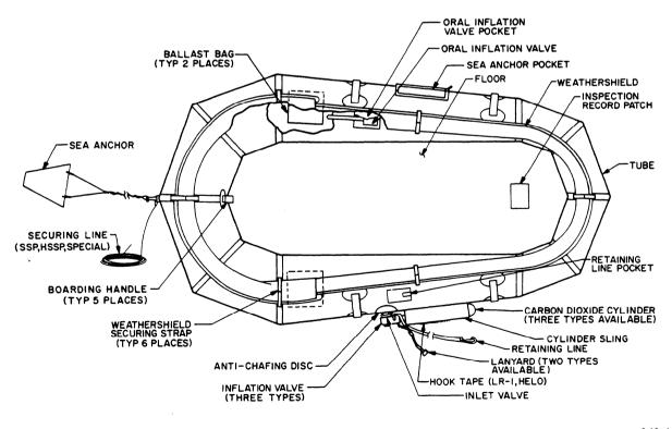
Figure 5-20.—LR-1 life raft assembly parts nomenclature.
