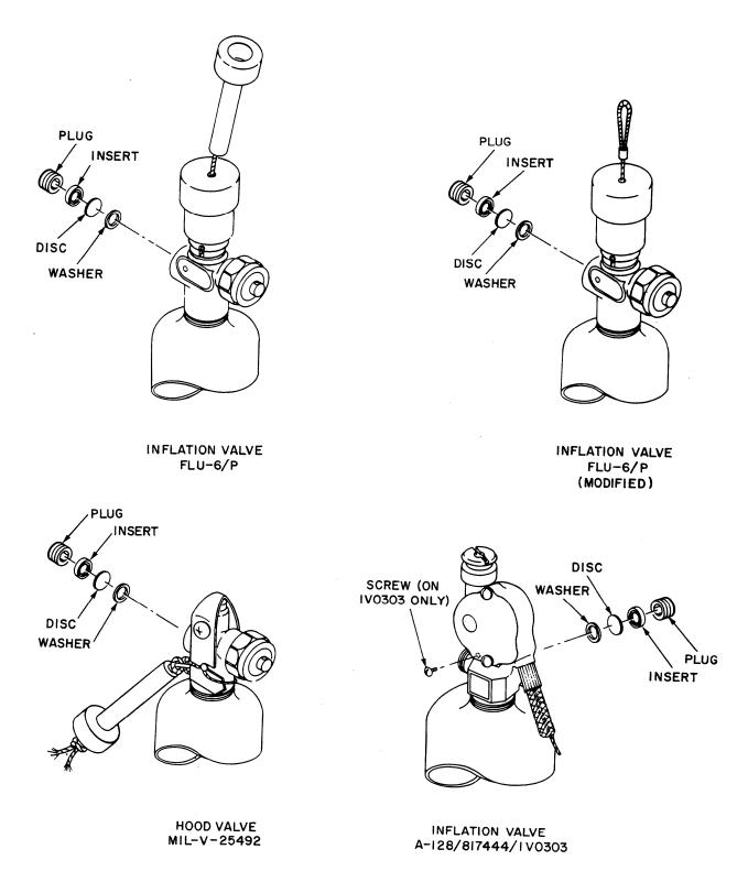
Figure 3-9.—Disassembly of Inflation Valve Safety Disc Assembly.
