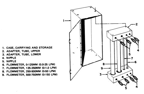
Figure 1-4.—Flowmeter Calibration Kit.
