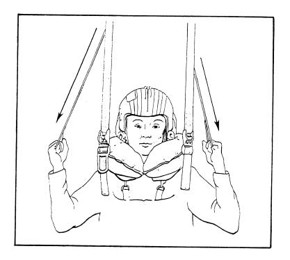
Figure 5-14.—Aircrewman pulling lanyard loops.
