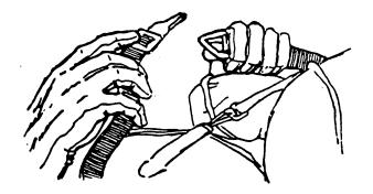
Figure 5-29.—Removing the pull tabs.
