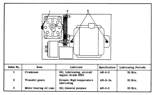
Figure 3-7.—Lubrication points.
