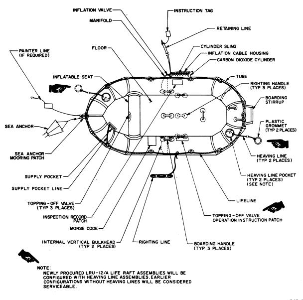
Figure 5-21.—LRU-12/A life raft assembly parts nomenclature.
