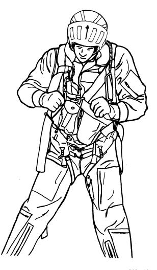
**240.113** Figure 5-5.—Aircrewman attaching quick release V-ring.
