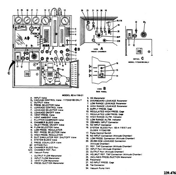
Figure 2-1.—Controls and indicators for oxygen system components test stand model 1172AS100.
