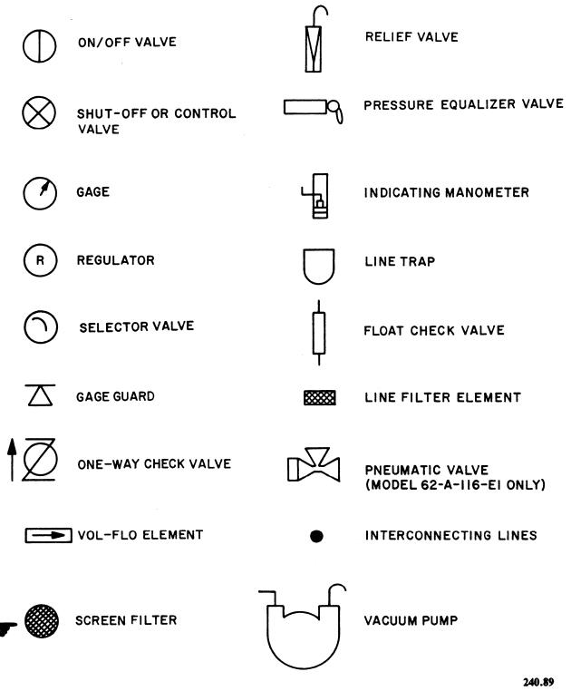
Figure 2-2.—Test stand schematic symbols.
