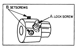
240.155 Figure 4-10A.—Presser-lifting eccentric connection link.
