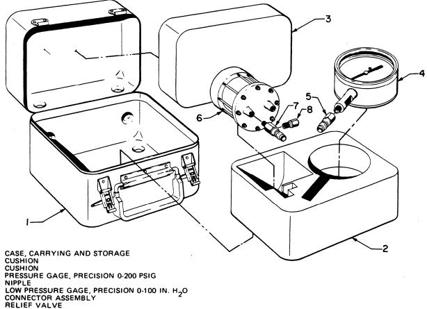
Figure 1-3.—Pressure Gage Calibration Kit.
