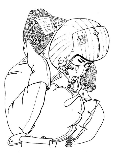
Figure 5-13.—Aircrewman releasing the hook-and-pile tapes on collar.
