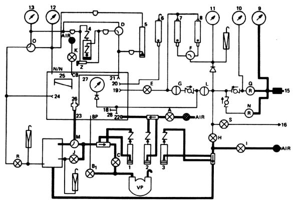
Figure 2-11.—Model 1172AS100 flow measuring system.
