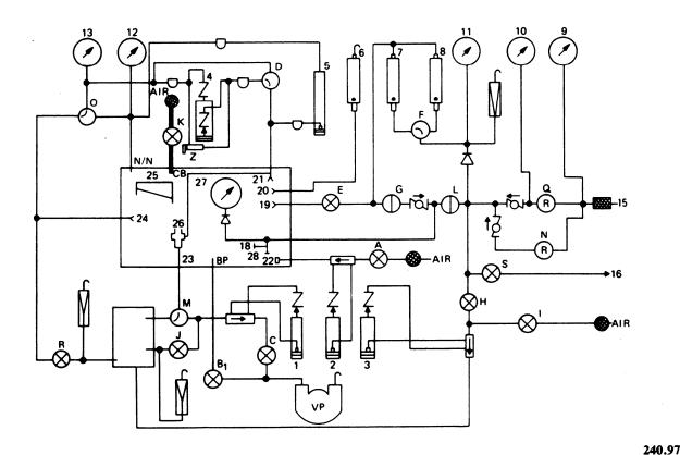
Figure 2-10.—Model 1172AS100 chamber bleed system.
