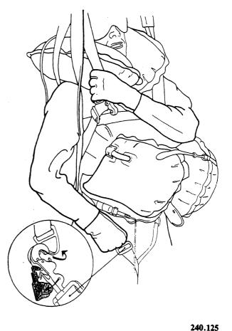
Figure 5-17.—Aircrewman releasing right leg strap quickejector snap.
