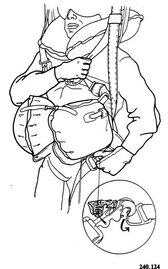
Figure 5-16.—Aircrewman releasing left leg strap quickejector snap.
