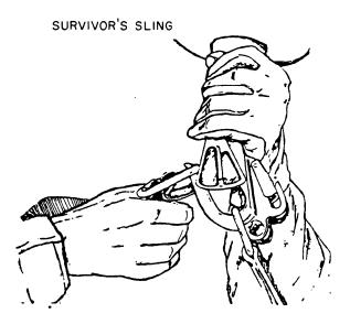
**240.133** Figure 5-25.—Attaching the rescue hook to the gated D-ring.
