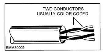
Figure 1-9.—Twisted-wire pairs (2 wire pairs shown).
