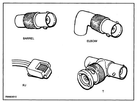
Figure 2-4.—Connector shapes.
