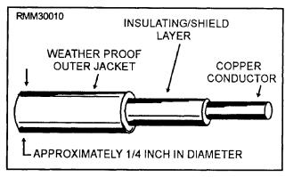
Figure 1-10.—Coaxial cable,
