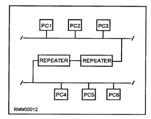
Figure 2-1.—Repeaters used to lengthen individual network segments.
