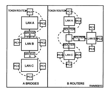
Figure 2-2.—Interconnecting LANS using (A) bridges and (B) routers.
