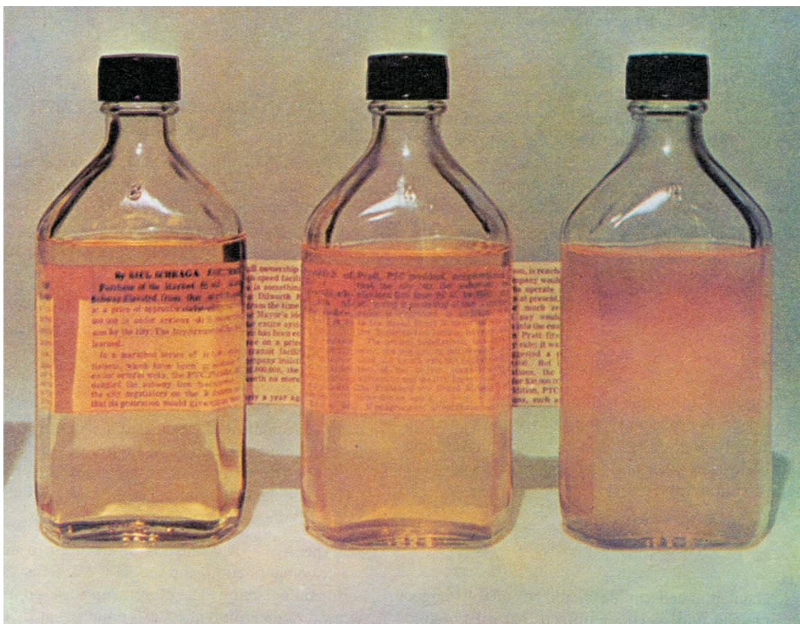
Figure 1-5.—Degrees of cloudiness in JP-5. The left sample is clean and bright and is the only acceptable fuel for aircraft.
