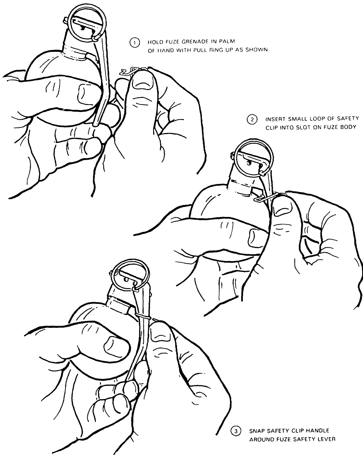
Figure 3-5. Assembly of safety clip to grenade M67.
