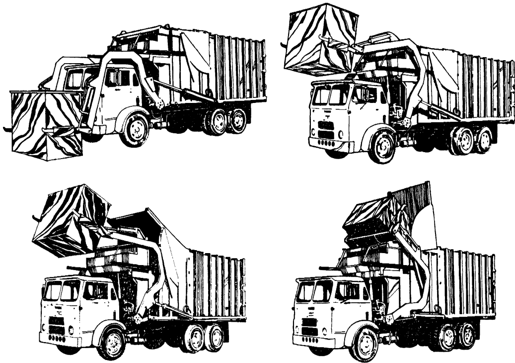
Figure 1-1. Front-loading compactor vehicle emptying a self-loading container.
