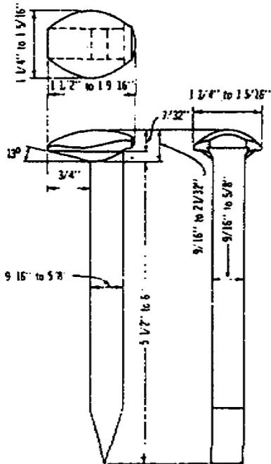
Figure 3.9. Details of Cut Spike.
