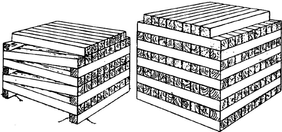
A. Method of stacking untreated ties
