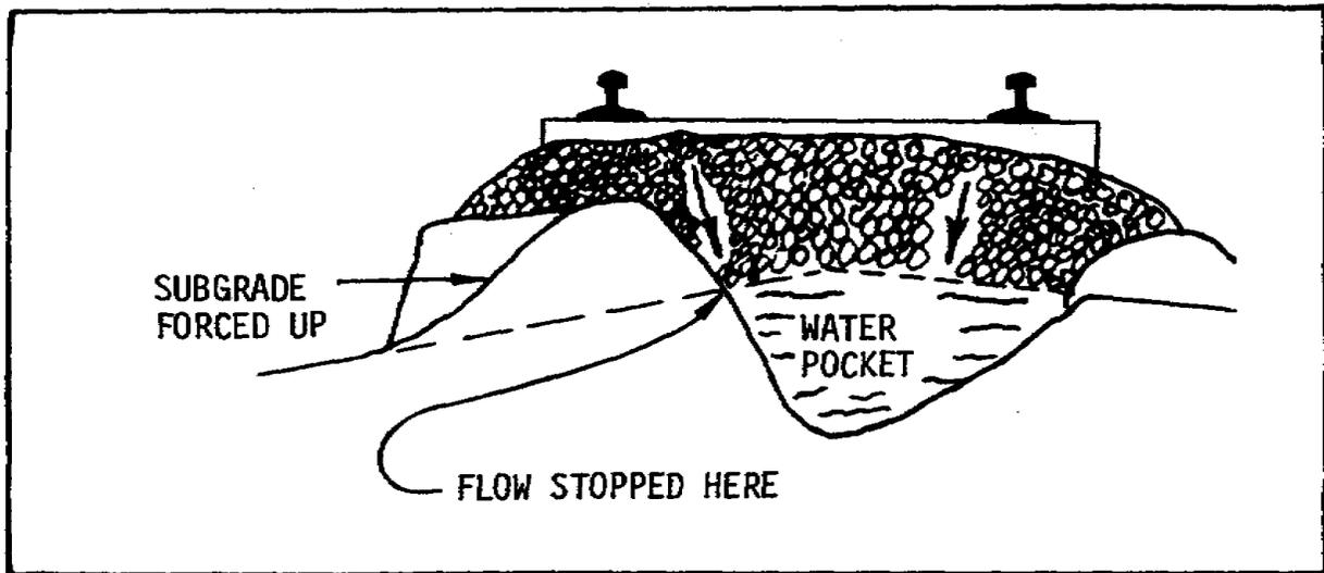
Figure 2.4. Drainage Obstructed When Subsoil Forced Up
