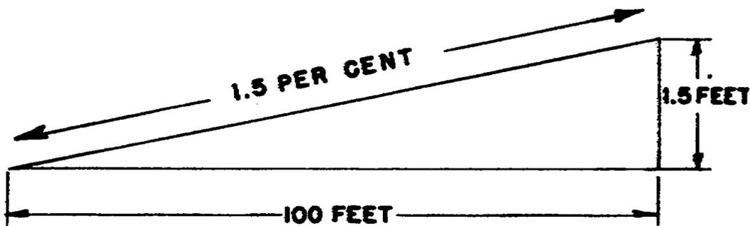
$$\begin{aligned}\text{PER CENT GRADE} &= \frac{1.5}{100} \times 100 \\ &= 1.5\end{aligned}$$
