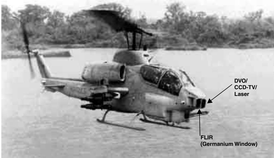
**Figure 3-6. AH-1W with the NTS.**
