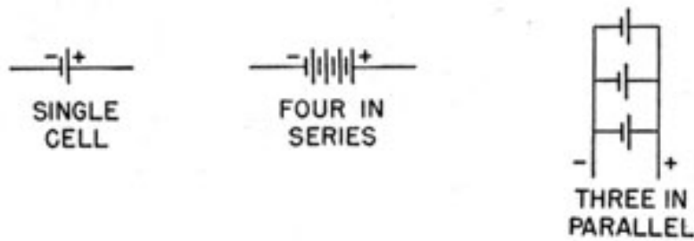
Figure 20.-Symbol for cells in series and parallel.
