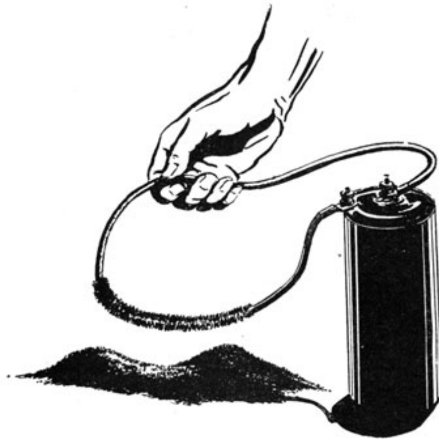
Figure 45.-Magnetism produced by a current.
