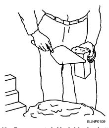
Figure 4-10.—Proper way to hold a brick when buttering the end.
