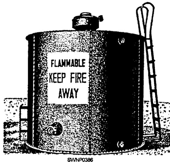
Figure 9-1.—100-barrel capacity, vertical, bolted steel tank.
