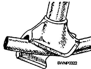
Figure 7-10.—Bending tool.
