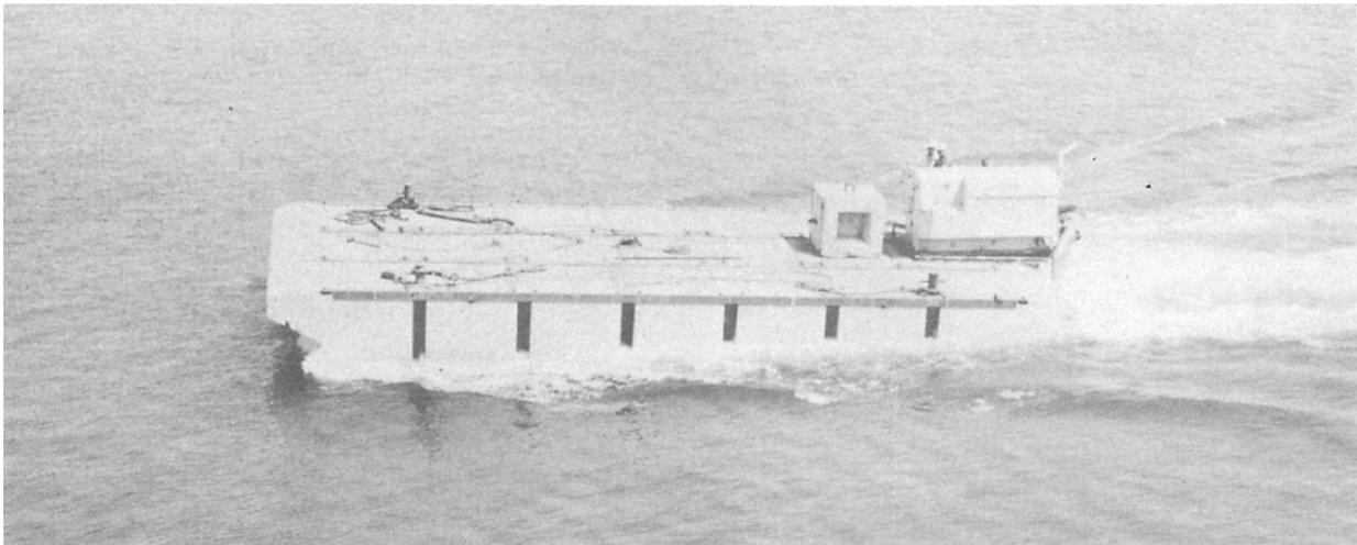
**Figure 10-27.—A 3x7 pontoon barge with a propulsion unit.**
