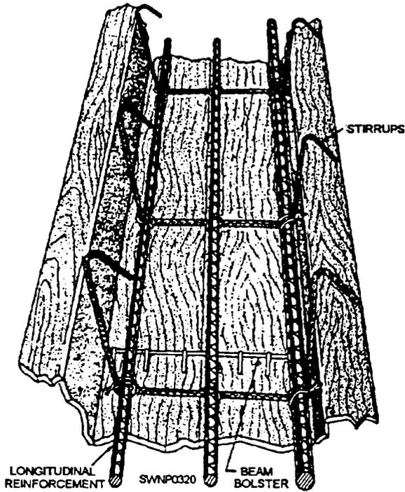
Figure 7-8.—Steel in place in a beam
