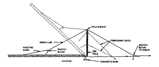
Figure 8-36.—Erection of a pivoted guyed tower.
