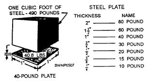
Figure 3-4.—Weight and thickness of steel plate.
