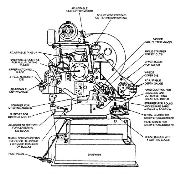
Figure 12-8.—Combination punch, shear, and coper.
