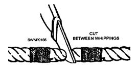
Figure 4-7.—Cutting a line between whipping.
