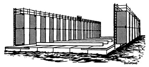
Figure 10-35.-6 x30, 400-ton pontoon dry dock.
