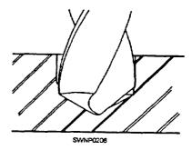
Figure 12-20.—Unequal drill point angles.
