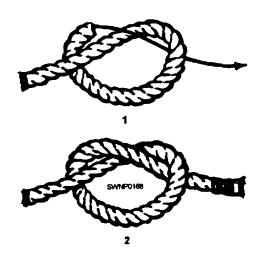
Figure 4-9.—Overhand knot.
