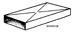
Figure 2-92.—Cross-broken flat surfaces
