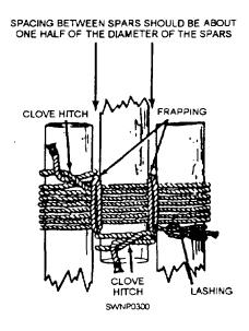
Figure 6-53.—Lashing for a tripod.
