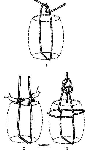
Figure 4-22.—A vertical barrel hitch.
