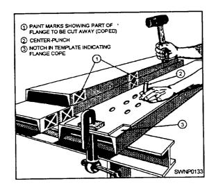
Figure 3-40.—Use of template in laying out a steel channel.
