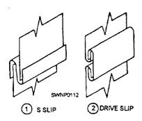
Figure 2-95.—Methods of connecting ducts,
