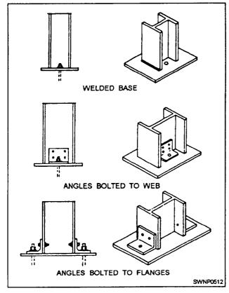
Figure 3-8.—Typical column to baseplate connections.
