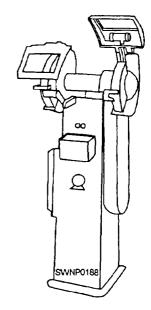
Figure 12-2.—The pedestal grinder (dry type).
