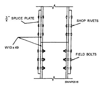
Figure 3-12.—Column splice with no size change.
