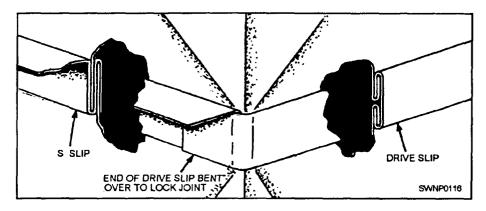
Figure 2-99.—Completed S-and-drive connection.
