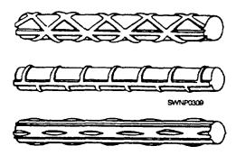
Figure 7-1.—Various types of deformed bars.
