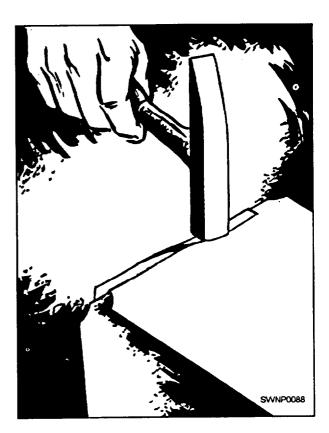
Figure 2-71.—Closing a Pittsburgh lock seam
