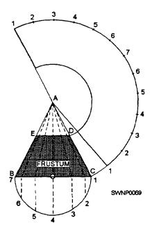
Figure 2-52.—Radial line development of a frustum of a cone.
