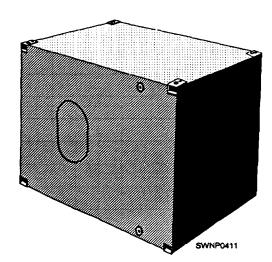
Figure 10-1.—P1 pontoon.
