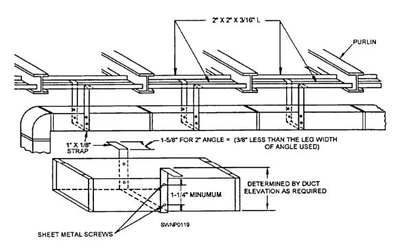
Figure 2-102.—Duct system with strap hangers from angle rails transverse to purlti
