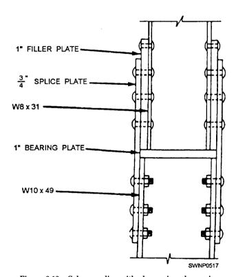
Figure 3-13.—Column splice with change in column size.
