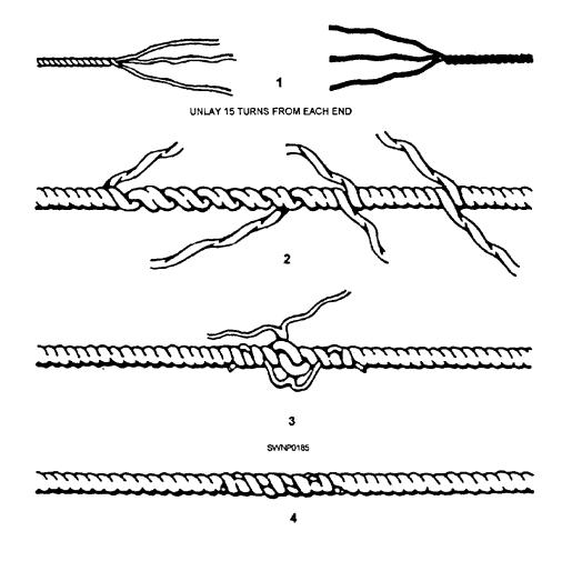
Figure 4-26.—Making a long splice.
