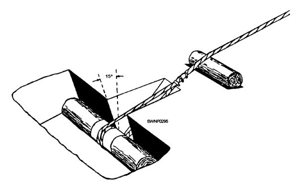
Figure 6-48.—A deadman anchorage for a heavy load.
