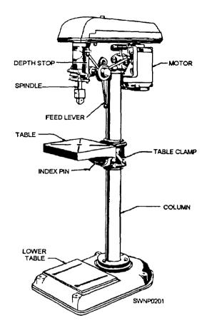
Figure 12-15.—Sensitive drill press.
