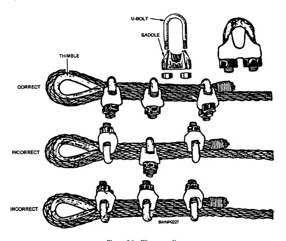
Figure 5-8.—Wire rope clips
