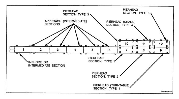
Figure 10-39.—Types and positions of causeway sections in the ELCAS.
