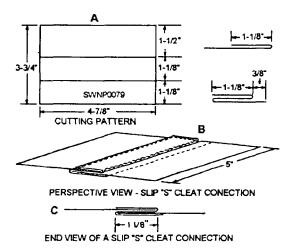
Figure 2-62.—"S" joint or slip pattern and connections.
