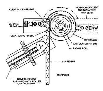
Figure 7-14.—Example of bending a 180-degree hook with No. 11 rebar.
