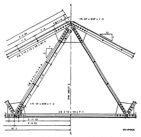
Figure 3-21.—Steel truss fabricated from angle-shaped members.
