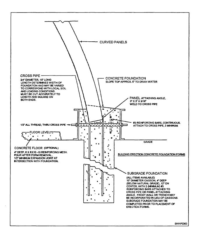
Figure 8-19.—Concrete foundation.
