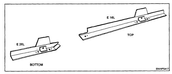
Figure 10-7.—Assembly angles E 16L and E 26L.
