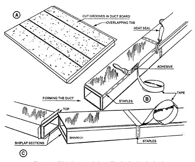
Figure 2-104.—Fabricating rectangular/square fiber-glass duct from duct board.
