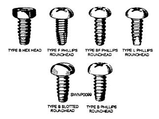
Figure 2-82.—Thread-cutting screws.
