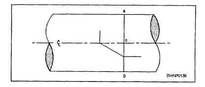
Figure 3-46.—Simple miter turn.
