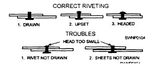
Figure 2-87.—Correct and incorrect riveting.
