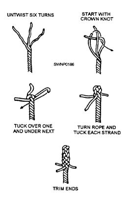
Figure 4-27.—Making a back splice
