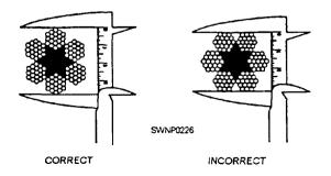
Figure 5-7.—Correct and incorrect methods of measuring wire rope.
