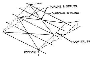
Figure 3-23.—Diagonal braces-top chord plane.
