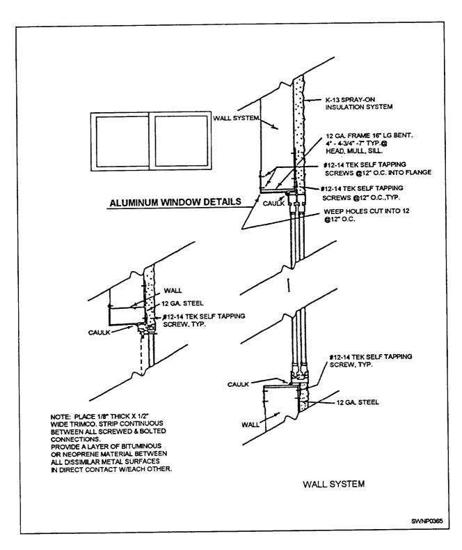
Figure 8-21.—Aluminum window installation.
