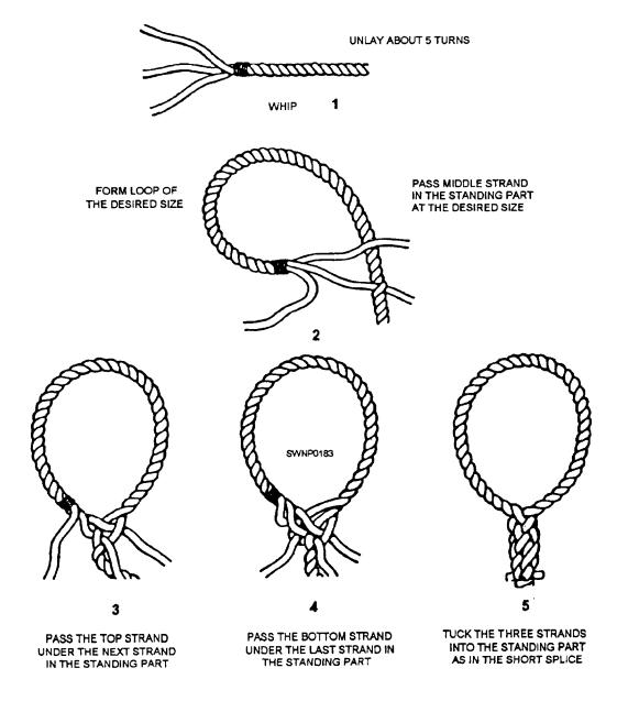
Figure 4-24.—Making an eye splice.
