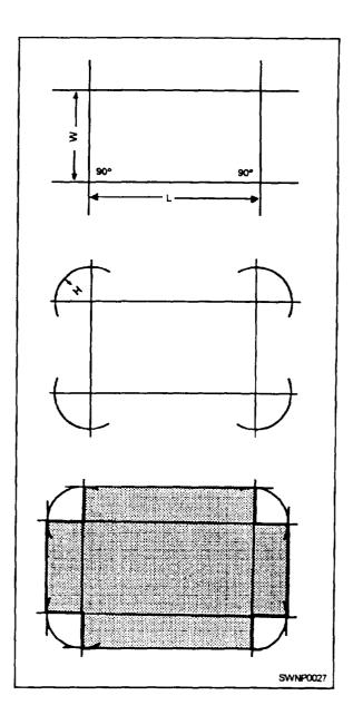
Figure 2-10.—Laying out a drip pan with dividers.
