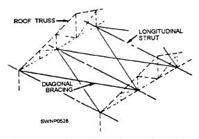
Figure 3-24.—Diagonal braces-bottom chord plane.
