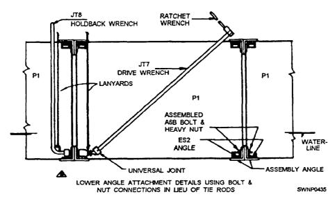
Figure 10-25.—Lower angle attachment details using bolt and nut connections instead of tie rods.
