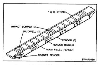
Figure 10-40.—ELCAS fender system details
