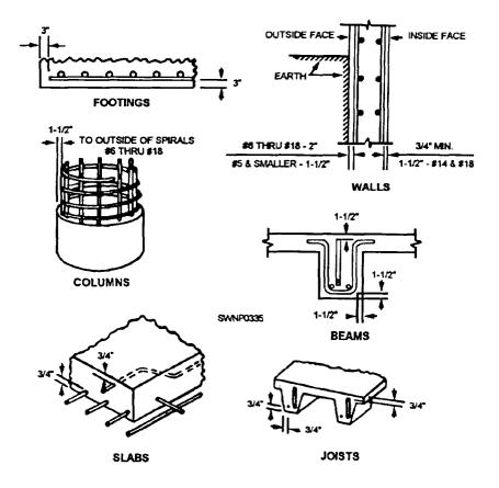
Figure 7-21.—Minimum coverage of rebar in concrete.
