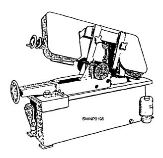
Figure 12-12.—Horizontal band Cutoff saw.
