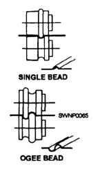
Figure 2-48.—Turning a bead with a rotary machine.
