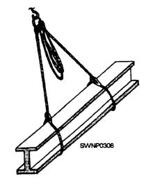
Figure 6-61.—Secure sling legs that are not used.
