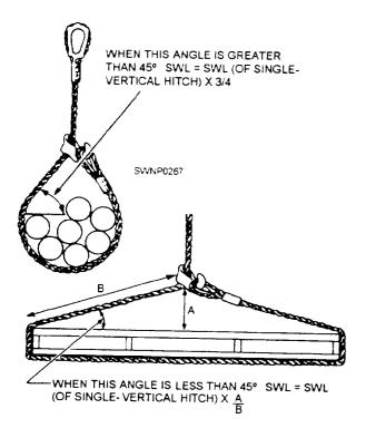
Figure 6-20.—Determination of single-choker hitch sling capacity.
