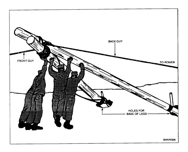
Figure 6-57.—Erecting shears
