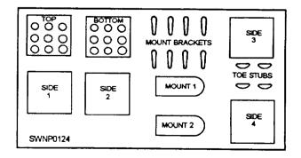
Figure 3-31.—Improper plate steel cooling box layout.
