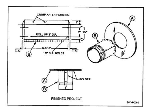
Figure 2-75.—Dovetail lock seam
