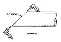
Figure 3-60.—Miter cutting.
