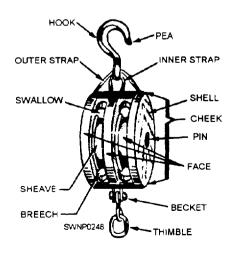
Figure 6-1.—Parts of a fiber line block.
