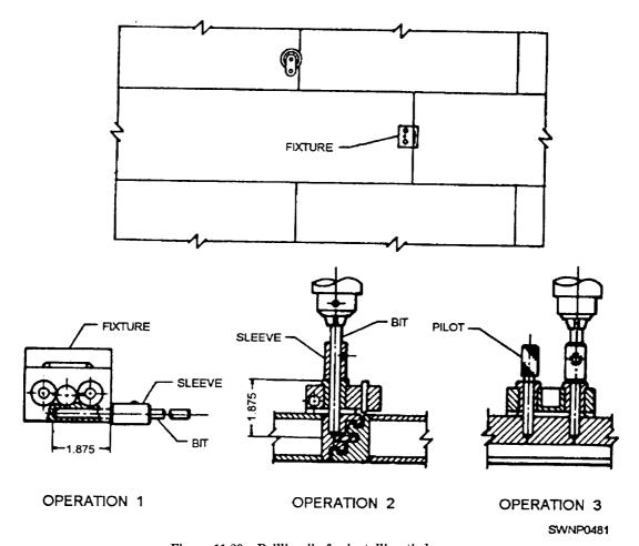
Figure 11-29.—Drilling jig for installing tiedowns
