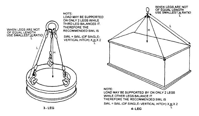
Figure 6-17.—Determination of bridle hitch sling capacity.
