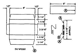
Figure 2-63.—Double "S' joint (cleat) pattern.
