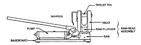
Figure 5-14.—Nicopress portable splicing tool.
