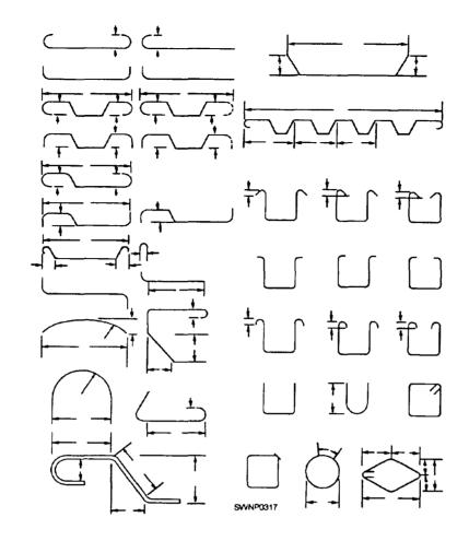
Figure 7-5.—Typical reinforcement bends.
