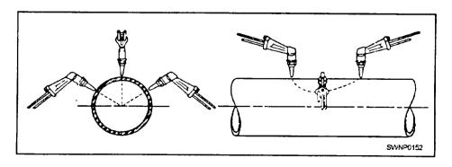
Figure 3-59.—Radial cutting.
