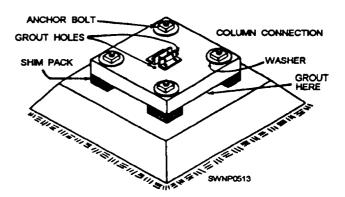
Figure 3-9.—Leveled bearing plate.
