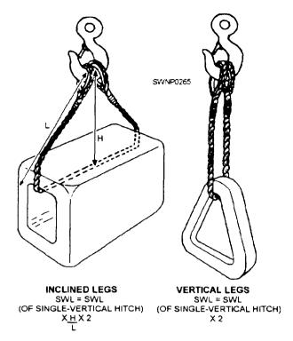
Figure 6-18.—Determination of single-basket hitch sting capacity.
