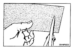
Figure 2-16.—Proper method of cutting with snips.
