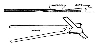
Figure 12-10.—Rejoining a broken band saw blade.
