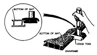
Figure 11-38.—Straightening of lower female edge.
