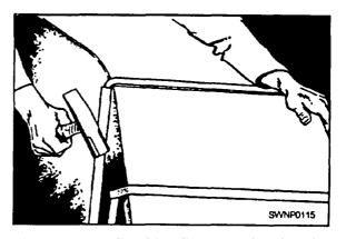
Figure 2-98.—Bending drive slips to complete the Joint.
