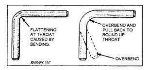
Figure 3-64.—Overbending to correct flattening of pipe.
