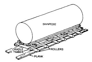
Figure 6-35.—Use of planks and rollers.
