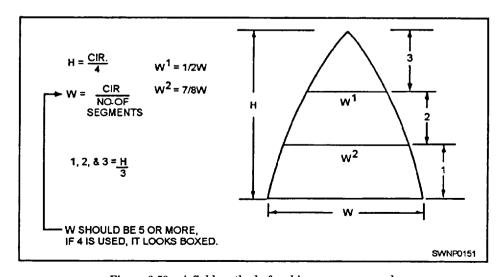
Figure 3-58.—A field method of making an orange peel.
