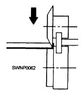
Figure 2-45.—Turning a burred edge.
