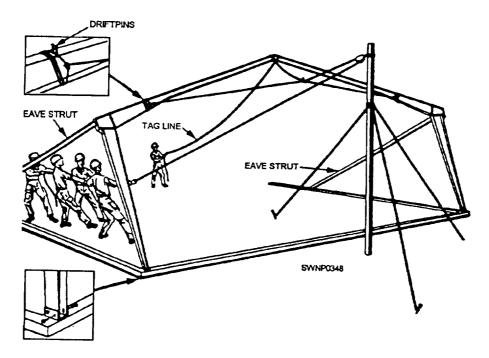
Figure 8-5.—Frame erection.
