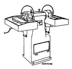
Figure 12-3.—Pedestal grinder (wet type) wttb a built-in coolant system
