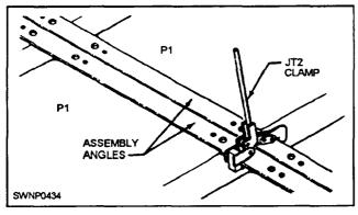
Figure 10-24.—Angle clamp for assembly of pontoon strings
