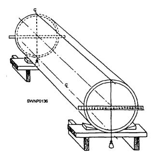
Figure 3-43.—Locating the top and the bottom center lines.
