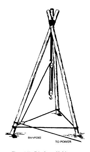
Figure 6-55.—Tripod assembled for use.
