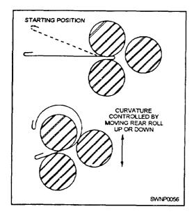
Figure 2-39.—Forming cylinders on rolling forms.
