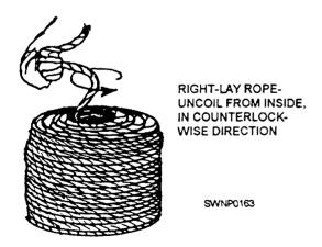
UNCOILING A NEW COIL OF FIBER ROPE
