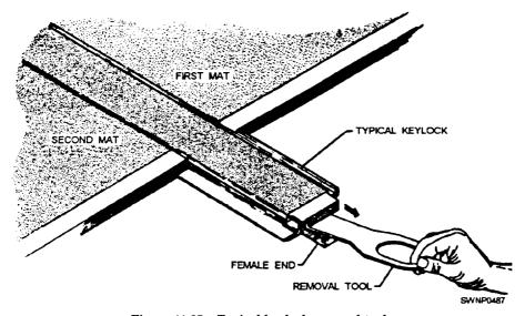
Figure 11-35.—Typical keylock removal tool.
