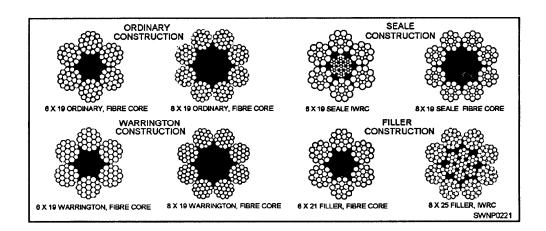
Figure 5-2.—Common strand construction.
