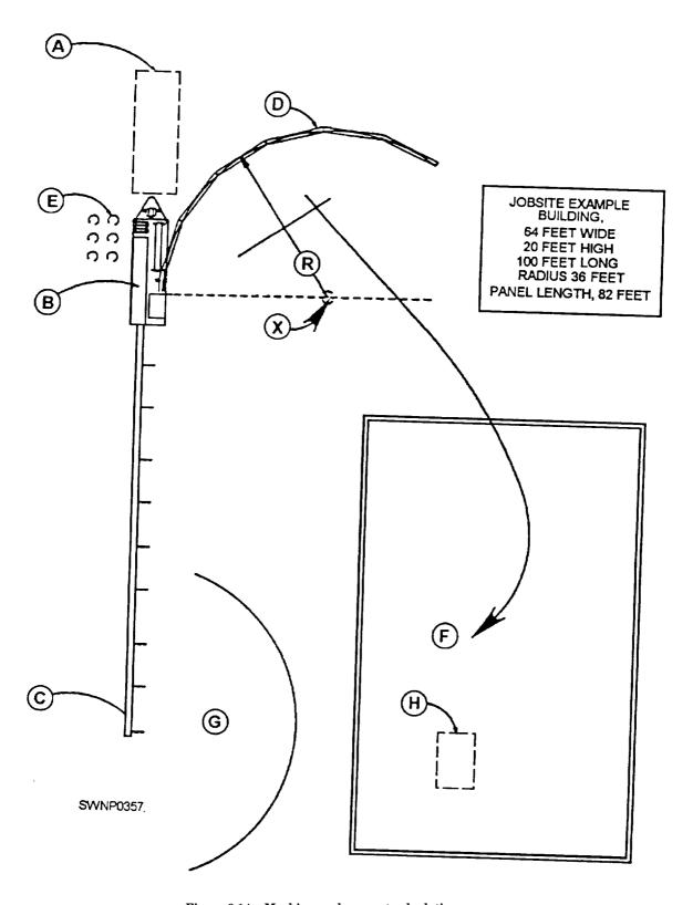
Figure 8-14.—Machinery placement calculations.
