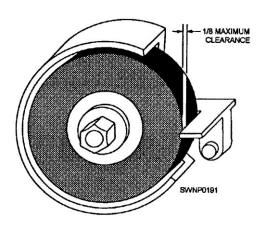
Figure 12-5.—Properly spaced tool rest.
