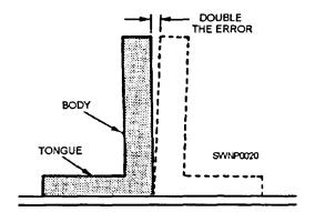
Figure 2-3.—Checking a square for accuracy.
