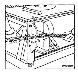
Figure 7-16.—Ironmaster bar-cutting unit.
