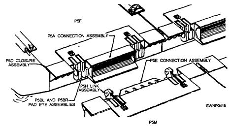
Figure 10-5.—End-to-end connections for P5M and P5F pontoons.
