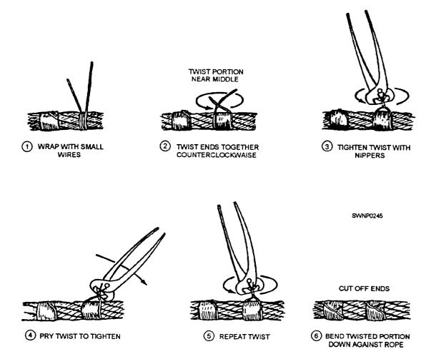
Figure 5-26.—Seizing wire rope.
