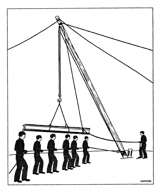
Figure 6-52.—Hoisting with a gin pole.
