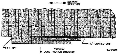
Figure 11-25.—Procedure No.1, 90-degree connectors.
