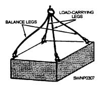
Figure 6-60.—Multi-legged bridle sling lifting a load.
