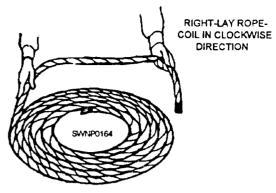
COILING OF A FIBER ROPE AFTER BEING USED
