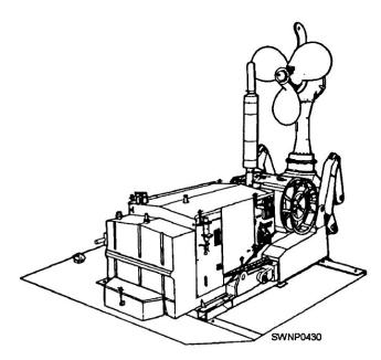
Figure 10-20.—Model L-295 diesel outboard propulsion unit.
