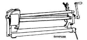
Figure 2-38.—Slip roll forming machine.
