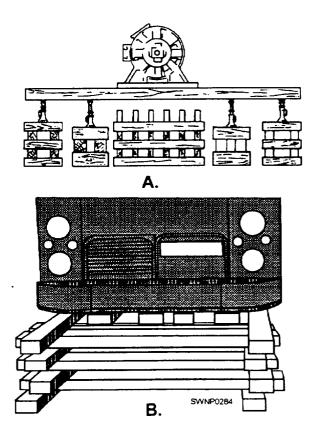
Figure 6-37.—Examples of the use of cribbing.
