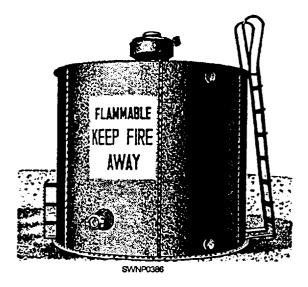
Figure 9-1.—100-barrel capacity, vertical, bolted steel tank.
