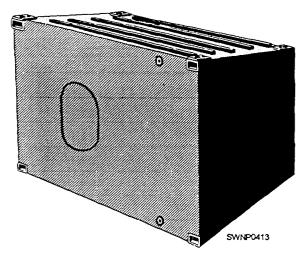
Figure 10-3.—P3 sloped deck pontoon,
