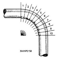
Figure 3-65.—90-degree bend made with ten separate wrinkles.
