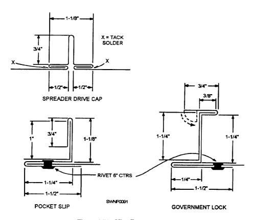
Figure 2-74.—Miscellaneous seam.
