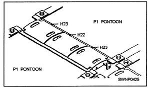
Figure 10-15.—Closure plates H22 and H23.
