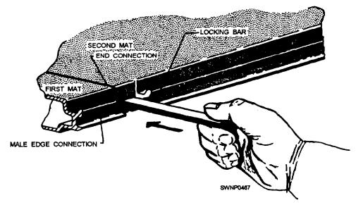
Figure 11-15.—Insertion of the locking bar.
