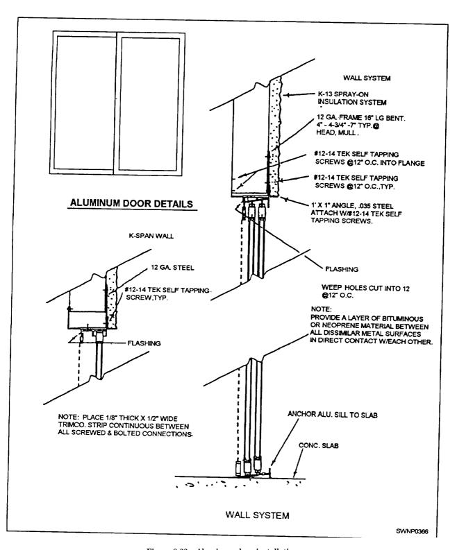
Figure 8-22.—Aluminum door installation.
