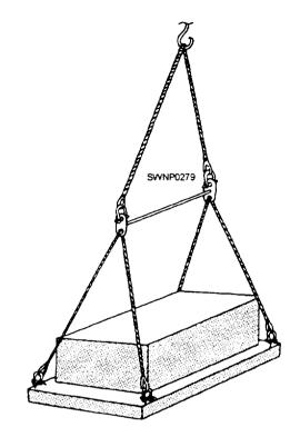
Figure 6-32.—Spreader bar used with an oversized load.
