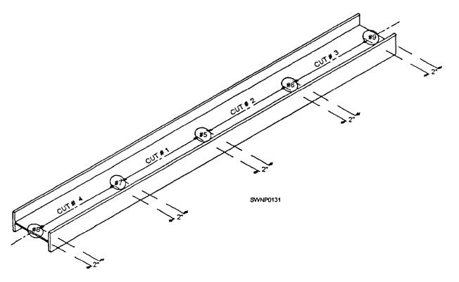
Figure 3-38.—Cutting order for splitting a beam.
