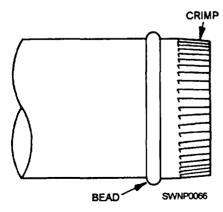
Figure 2-49.—A crimped section.
