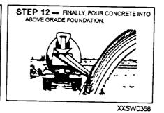
Figure 8-24.—Steps in K-span construction.
