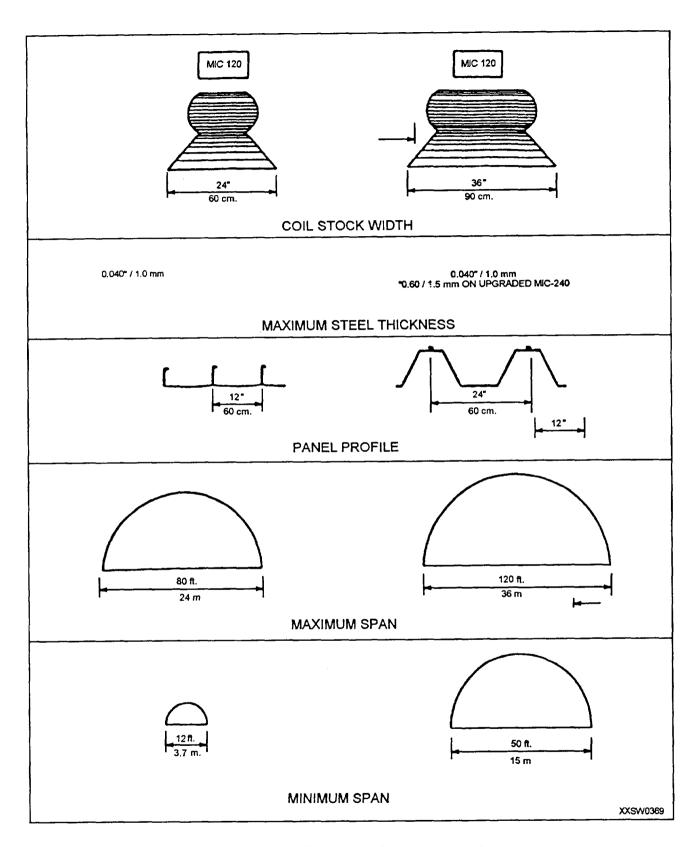
Figure 8-25.—ABM System 120 and 240 comparison chart.
