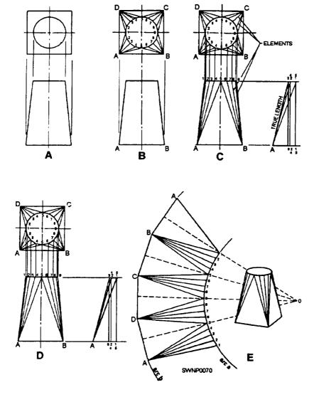
Figure 2-53.—Traingular development of a transition piece.
