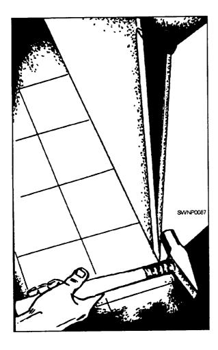
Figure 2-70.—Assembly of a Pittsburgh lock seam
