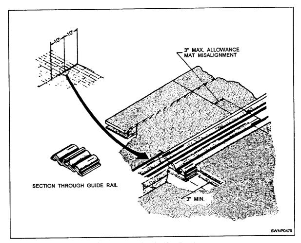
Figure 11-23.—Laying of guide rails and mats.
