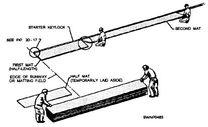
Figure 11-11.—Placing first and second mats
