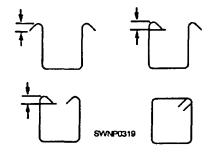
Figure 7-7.—Stirrup and column ties.
