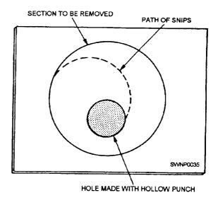
Figure 2-18.—Making an internal circular cut.
