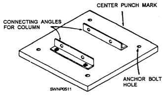
Figure 3-7.—Column bearing plate.
