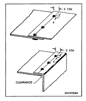
Figure 2-67.—Layout of lap seams for riveting.
