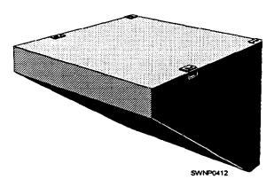
Figure 10-2.—P2 straight-line sloping bow pontoon.
