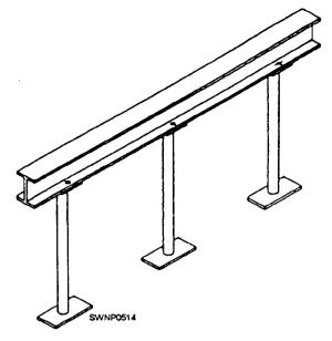
Figure 3-10.—Girder span on pipe columns.
