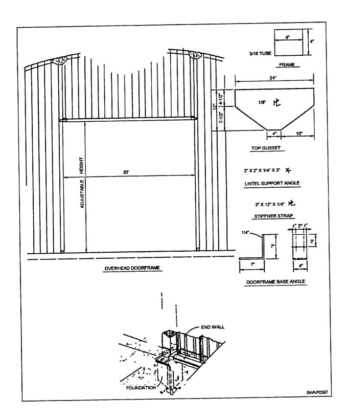
Figure 8-23.—Overhead doorframe.
