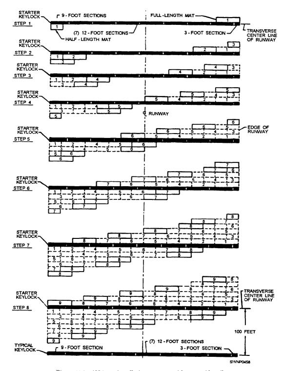
Figure 11-6.—AM-2 mat installation sequence without a guide rail.
