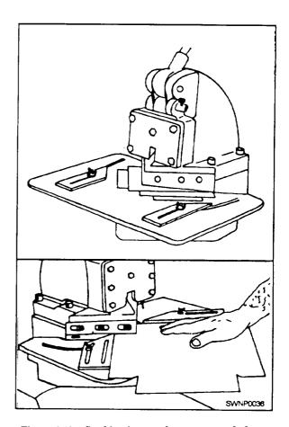
Figure 2-19.—Combination notcher, coper, and shear.
