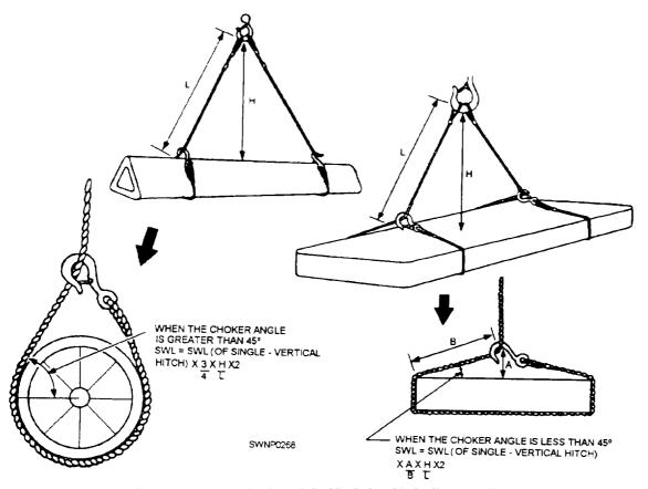
Figure 6-21.—Determination of double-choker hitch sling capacity.
