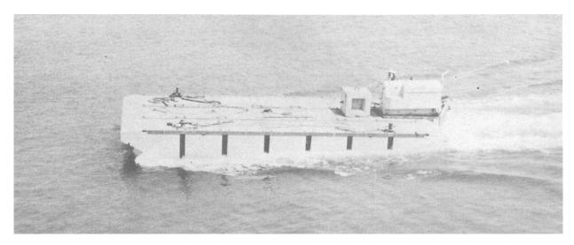
Figure 10-27.—A 3x7 pontoon barge with a propulsion unit.
