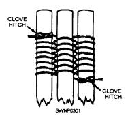
Figure 6-54.—Alternate lashing for a tripod.
