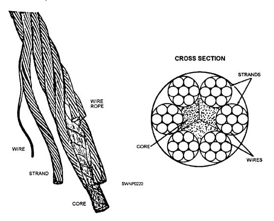
Figure 5-1.—Fabrication of wire rope
