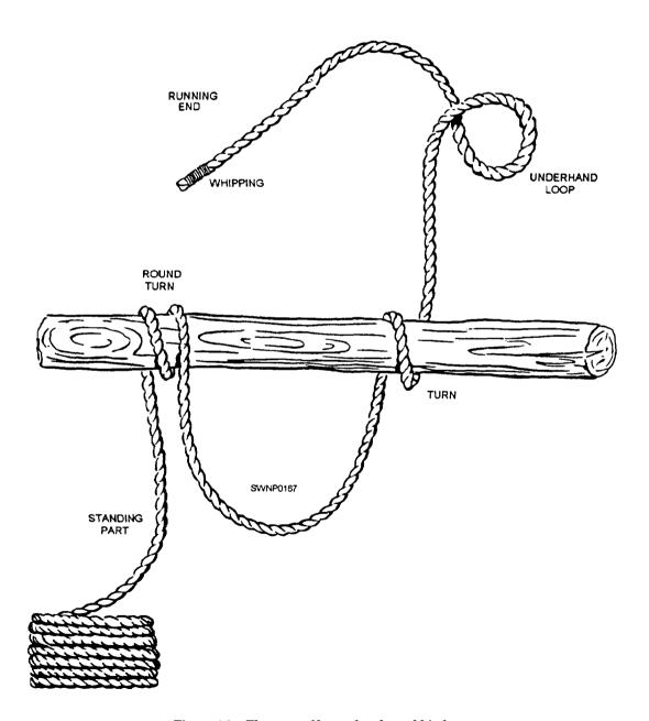
Figure 4-8.—Elements of knots, bends, and hitches
