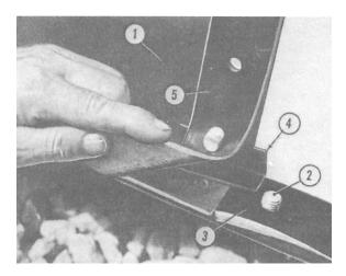
Figure 9-12.—Installing first stave.
