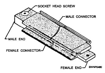
Figure 11-8.—Typical keylock.
