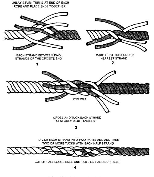
Figure 4-25.—Making a short splice.
