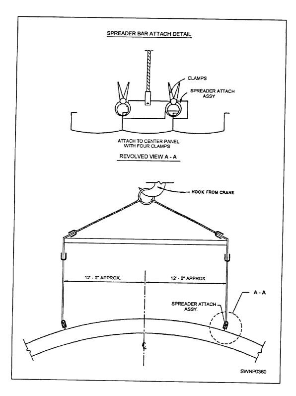
Figure 8-16.—Spreader bar attachment.
