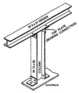
Figure 3-14.—Girder span on a wide flange column.
