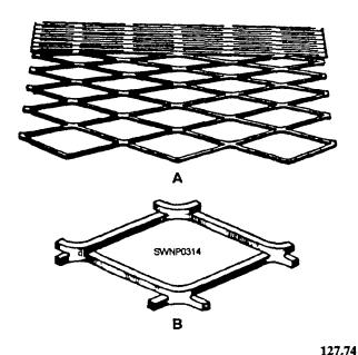
Figure 7-3.—Expanded or diamond mesh steel reinforcement.
