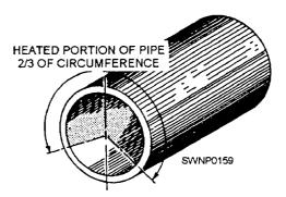
Figure 3-66.—Part of pipe heated before wrinkle bending.
