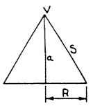
The stretchout of a right circular cone will be a portion of a circle whose radius (S) is equal to the slant height of the cone.
