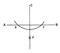
Step 1. From C, draw an arc using any convenient radius, intersecting AB at X and Y.
