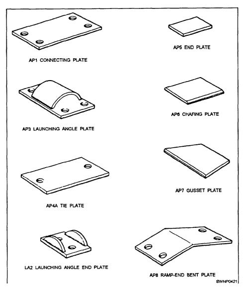
Figure 10-11.—Assembly plates.
