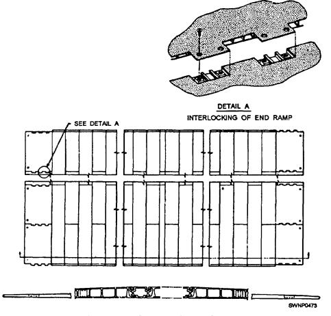
Figure 11-21.—Placement of mat end ramps.
