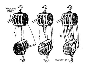
Figure 6-6.—Reeving two 3-sheave blocks.
