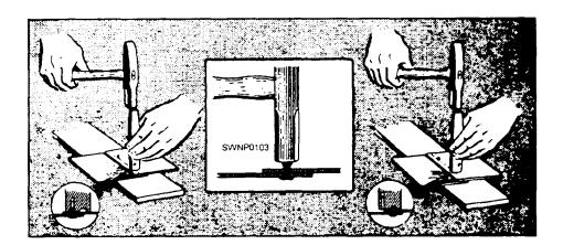
Figure 2-86.—Drawing, upsetting, and heading a rivet.
