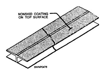
Figure 11-24 .- 90-degree connector.
