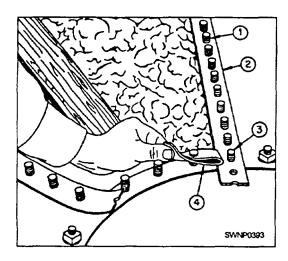
Figure 9-8.—Installation of bottom plates.
