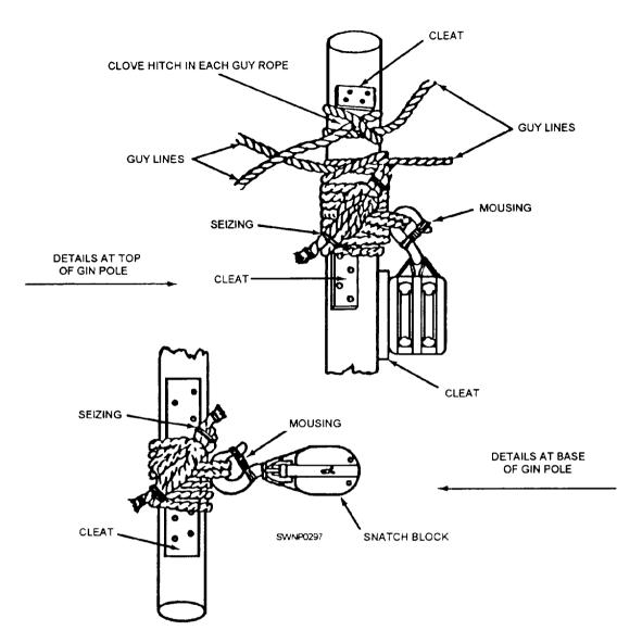
Figure 6-50.—Lashing for a gin pole.
