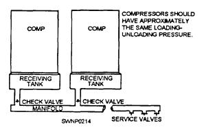
Figure 12-28.—Methods of manifolding compressors.
