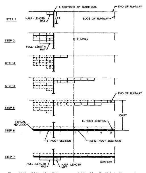
Figure 11-22.—AM-2 mat installation sequence (with guide rails—96-foot-wide runway).
