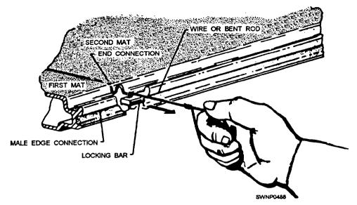
Figure 11-36.—Removal of locking bar.
