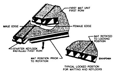
Figure 11-12.—Engaging first half mat (half length) to starter keylock.
