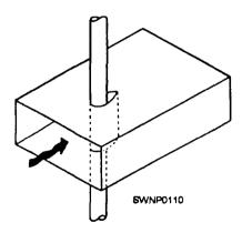
Figure 2-93.—Easement around an obstruction in ducts.
