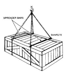
Figure 6-31.—Using spreader bars.
