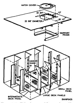
Figure 10-13.—H6 hatch cover and floor panel assembly.
