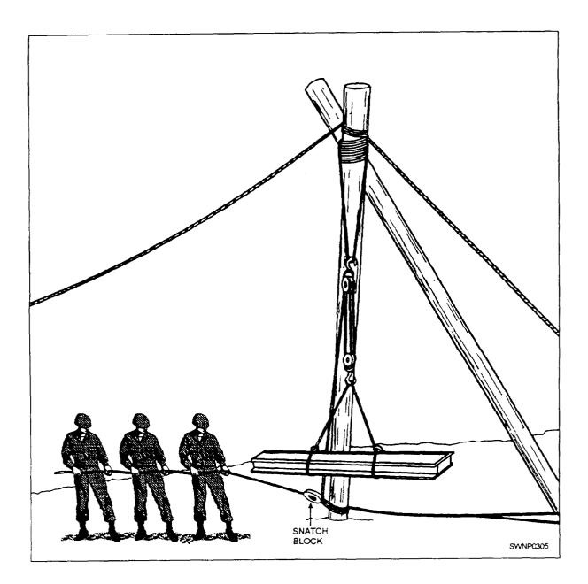
Figure 6-58.—Hoisting with shears.
