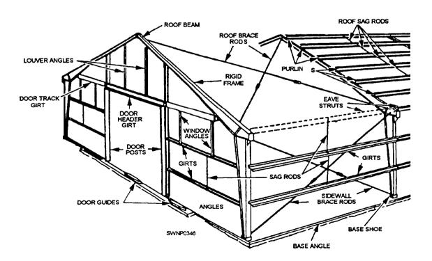
Figure 8-3.—Structural members of a pre-engineered building.
