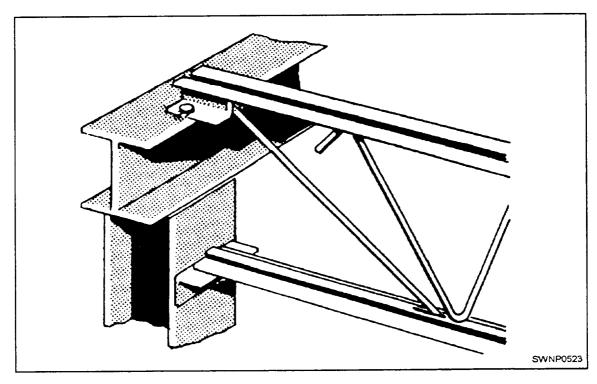
Figure 3-19.—Bar joists seat connection.
