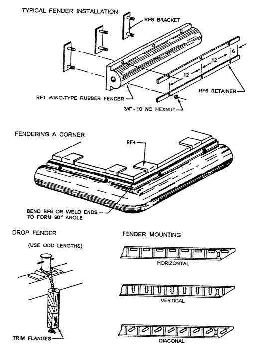
Figure 10-12.—Typical fender installations.
