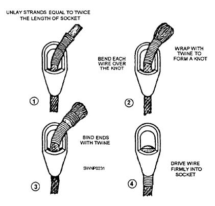
Figure 5-12.—Attaching a basket socket by the dry method.
