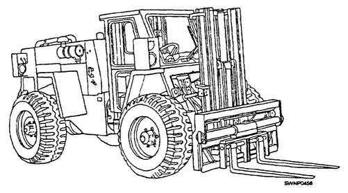
Figure 11-4.—4K rough-terrain forktlift.
