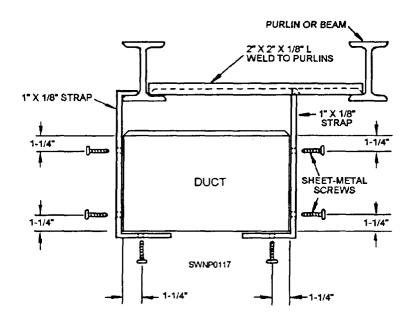
Figure 2-100.—Duct running parallel to purlins or beams.
