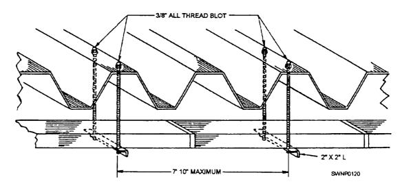
Figure 2-103.—Duct installed to a built-up steel roof.
