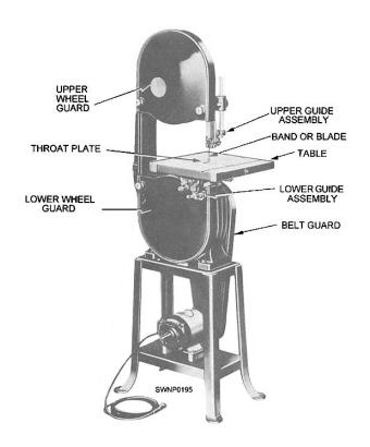
Figure 12-9.—14-inch band saw.
