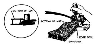
Figure 11-39.—Straightening of upper female edge.
