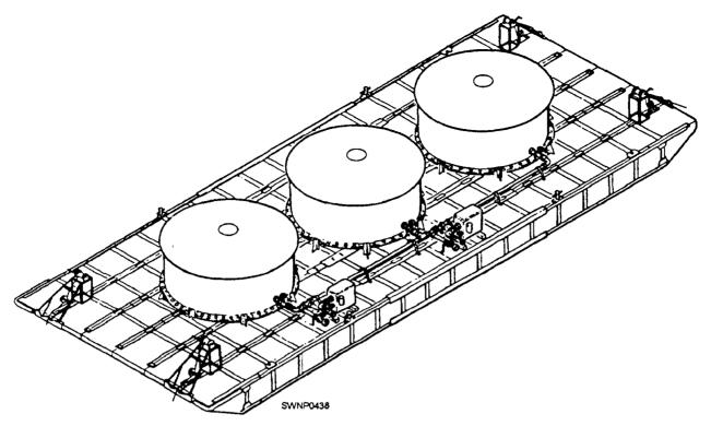
Figure 10-28.—A 1500 barrel, 6x18 fuel storage barge.
