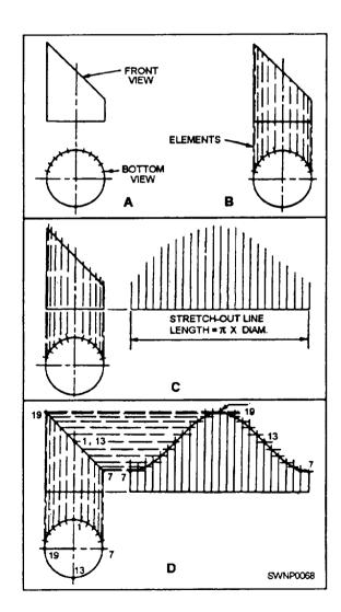
Figure 2-51.—Development of a truncated cylinder.
