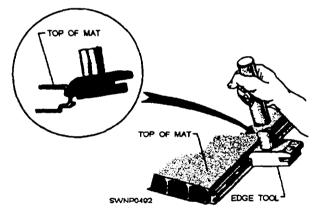
Figure 11-40.—Straightening of male edge.
