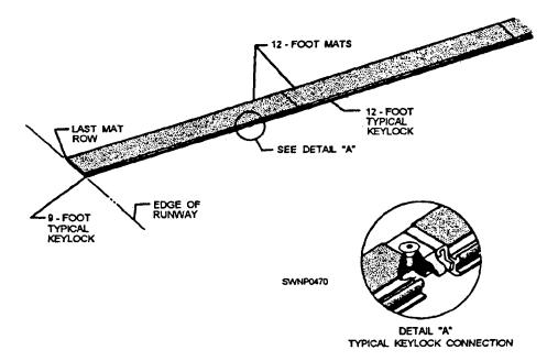
Figure 11-18.-Placing typical keylocks in a matting field.
