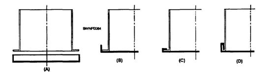
Figure 2-47.—Making a double seam on a cylindrical section.
