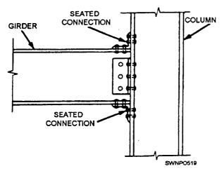
Figure 3-15.—Seated connections.
