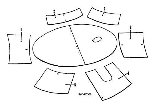
Figure 9-3.—Layout of the staves around the tank bottom.
