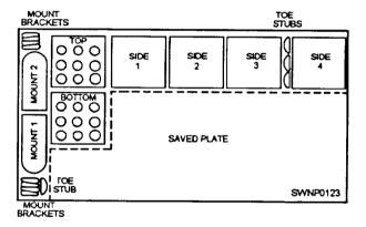
Figure 3-30.—Proper plate steel cooling box layout.
