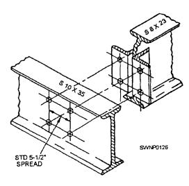
Figure 3-33.—Typical framed construction, top flange flush.
