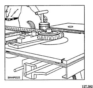
Figure 7-13.—Ironmaster bar-bending unit.
