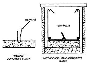
Figure 7-19.—Precast concrete block used for rebar support.
