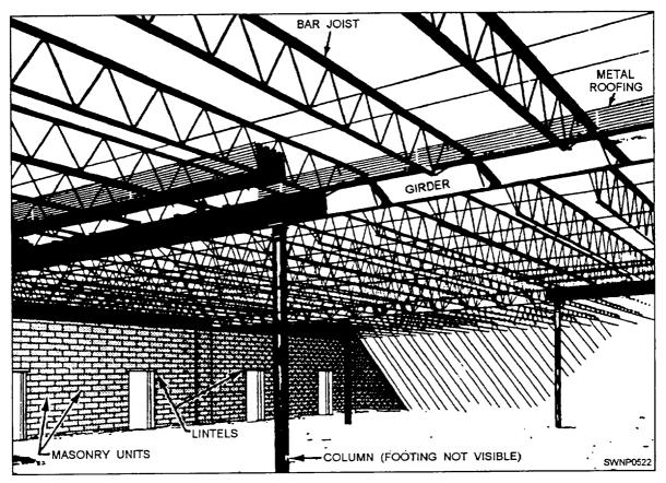
Figure 3-18.—Clearspan bar joists (girder to girder) ready to install roof sheeting.
