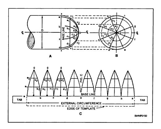
Figure 3-57.—Orange peel head.
