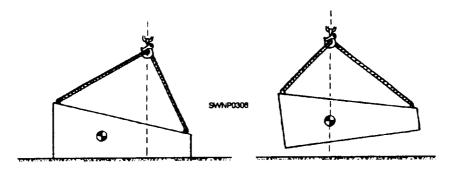
Figure 6-59.—Example of a load shifting when lifted.
