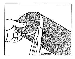
Figure 2-17.—Making a circular cut.
