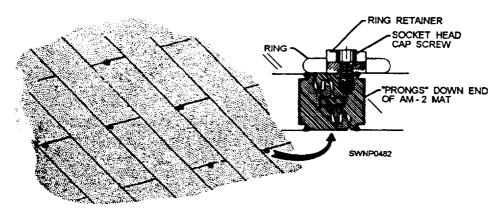
Figure 11-30.—Installing tie-downs in AM-2 matting.
