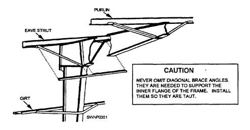
Figure 8-8.—Diagonal brace angles
