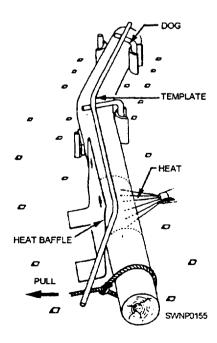
Figure 3-62.—Bending on a slab.
