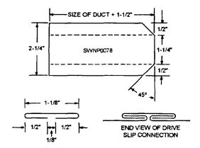
Figure 2-61.—Drive slip pattern and connections
