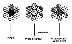
Figure 5-3.—Core construction.
