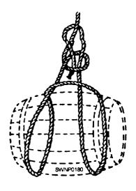
Figure 4-21.—Barrel hitch.
