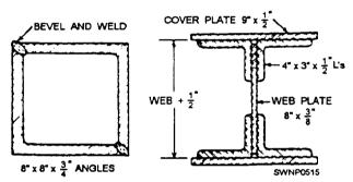
Figure 3-11.—Built-up column section.
