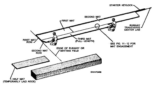
Figure 11-16.—Placing of third mat (full-length).
