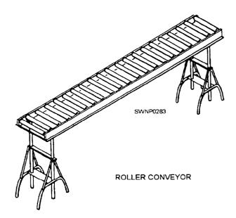
Figure 6-36.—Permanent metal roller conveyor.
