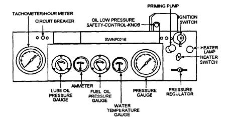
Figure 12-30.—Instrument panel.
