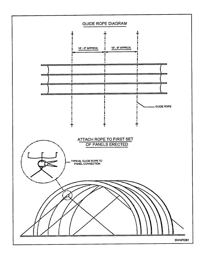
Figure 8-17.—Guide rope diagram.
