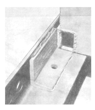
Figure 10-21.—Pontoon positioned on assembly angle.
