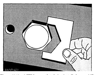
Figure 10-10.—A KPl keeper plate being installed on an A6B bolt.
