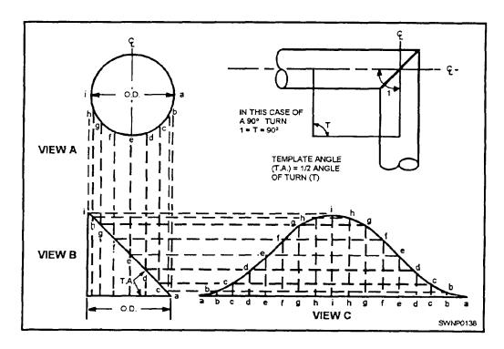
Figure 3-45.—Principles of template layout.
