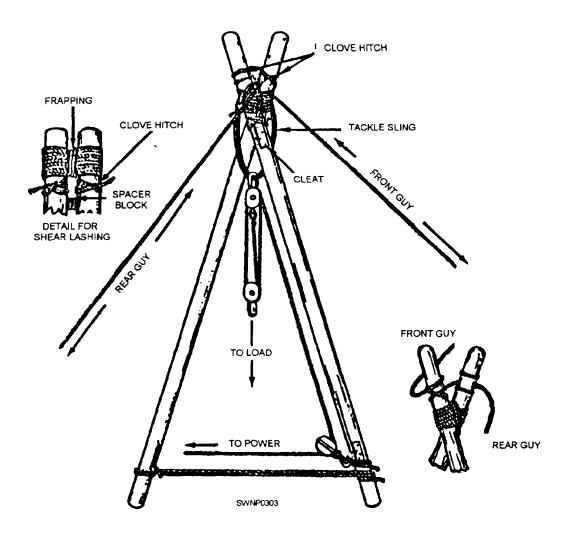
Figure 6-56.—Lashing for shears.
