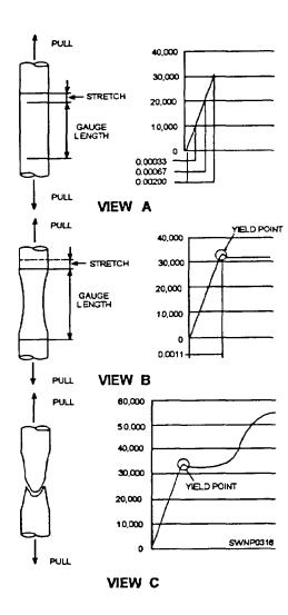
Figure 7-4.—Tension in steel bars.
