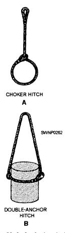
Figure 6-15.—Methods of using single-leg slings.
