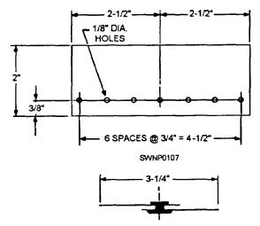
Figure 2-90.—Pattern for riveted lap seam.
