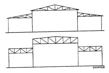
Figure 3-22.—Different styles of truss shapes.
