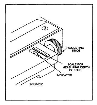
Figure 2-33.—Fold size depth gauge.
