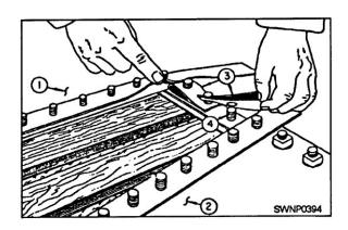
Figure 9-9.—Method of installing the wedge gaskets at the installation of the last bottom plate
