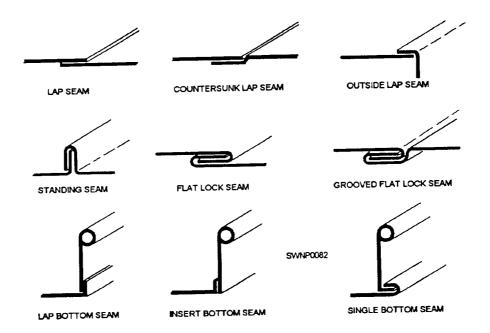
Figure 2-65.—Common sheet-metal seams.
