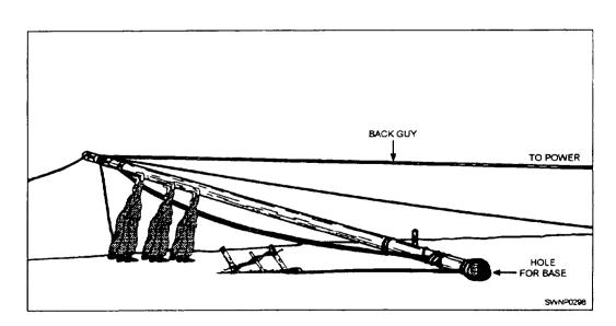
Figure 6-51.—Erecting a gin pole.
