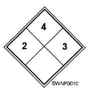
Figure 1-10.—Hazard warning lahel for methyl ethyl ketone.
