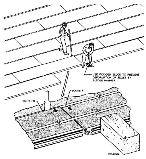
Figure 11-17.—Correction of mat misalignment.
