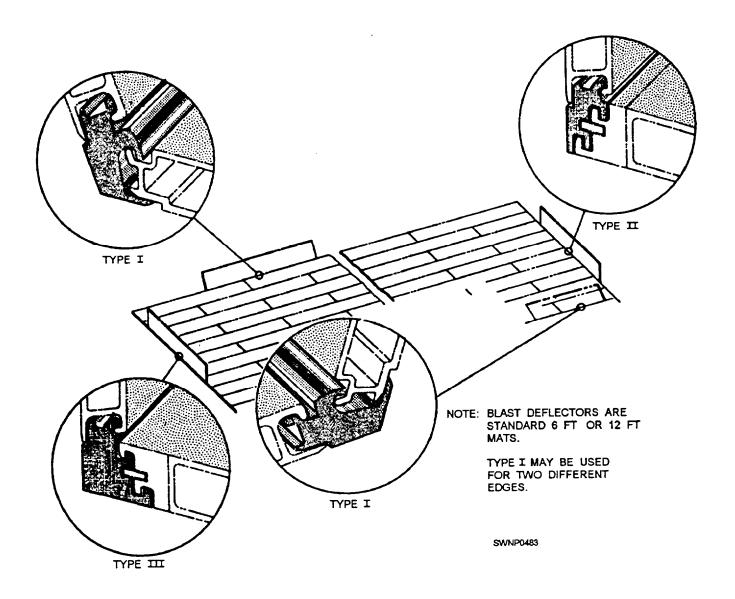
Figure 11-31.—Installation of blast deflector (adapters and mats).
