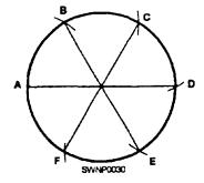
Figure 2-13.—Dividing a circle into six equal parts
