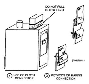
Figure 2-94.—Flexible duct connection.
