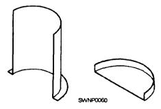
Figure 2-43.—Burrs turned on a cylindrical section.
