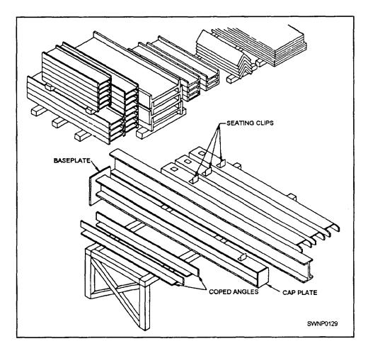
Figure 3-36.—Prefab table and steel storage.
