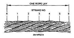
Figure 5-5.—Lay length of wire rope.
