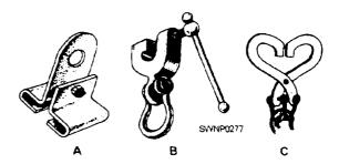
Figure 6-30.—Types of beam clamps.
