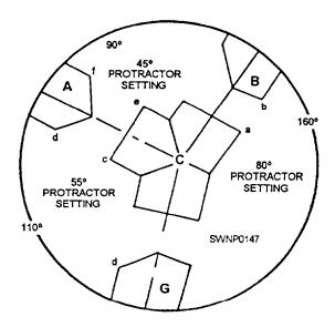
Figure 3-54.—Three-piece Y connection.
