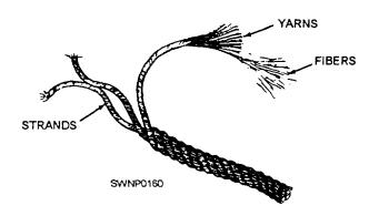
Figure 4-1.—Fabrication of line.
