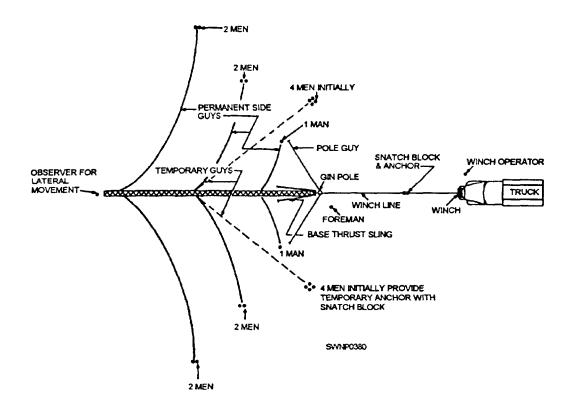
Figure 8-35.—Erection plan for a pivoted tower.
