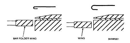
Figure 2-34.—Wing setting determines the tightness of fold.
