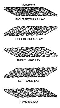
Figure 5-4.—Lays of wire rope.
