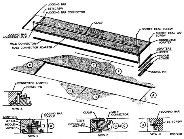
Figure 11-34.—Replacement mat installation.
