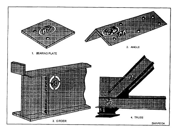
Figure 3-41.—Erection and assembly marks.
