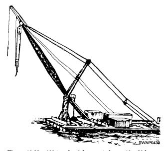
Figure 10-29.—100-ton derrick mounted on a 10 x 30 barge.
