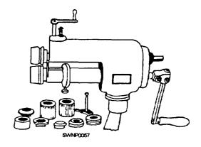
Figure 2-40.—Combination rotary machine with extra forming rolls.
