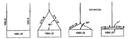
Figure 6-22.—Stress on slings at various vertical angles.
