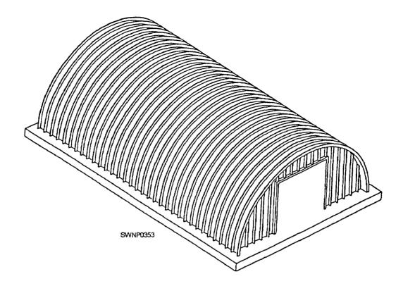
Figure 8-10.—Typical K-span building.
