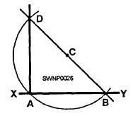
Figure 2-9.—Constructing a 90-degree angle at a given point
