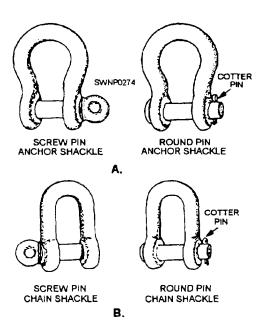
Figure 6-27.—Two types of shackles: A. Anchor; B. Chain.
