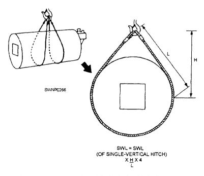
Figure 6-19.—Determination of double-basket hitch sling capacity.
