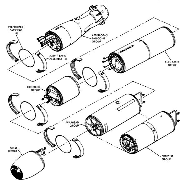
Figure 3-4.-Mk 48 torpedo group configuration.
