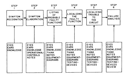
Figure 5-13.-Six-step procedure.
