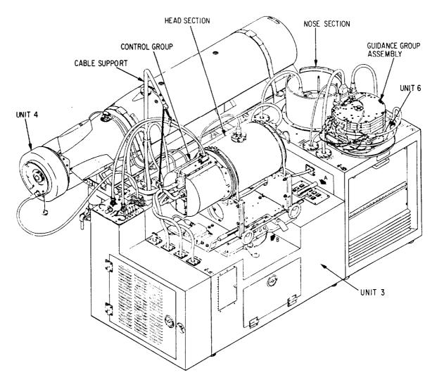
Figure 2-30.-Guidance and control test fixture, unit 3.
