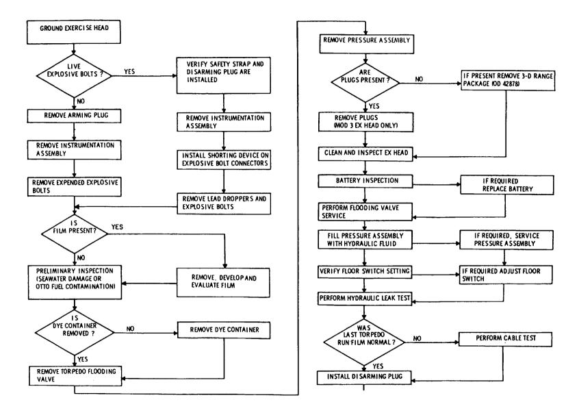
Figure 2-18.-Maintenance flow diagram for the exercise head.
