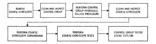
Figure 2-20.-Control group turnaround diagram.
