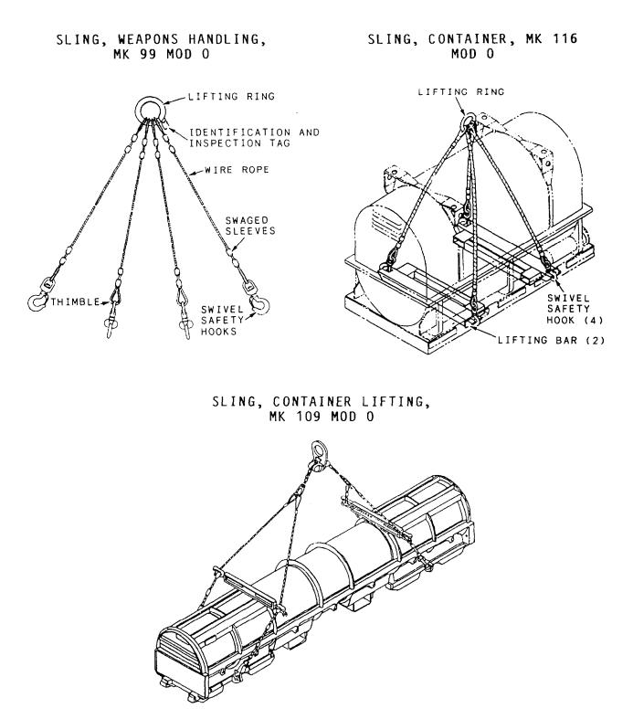
Figure 1-15.-Slings for lifting containers.
