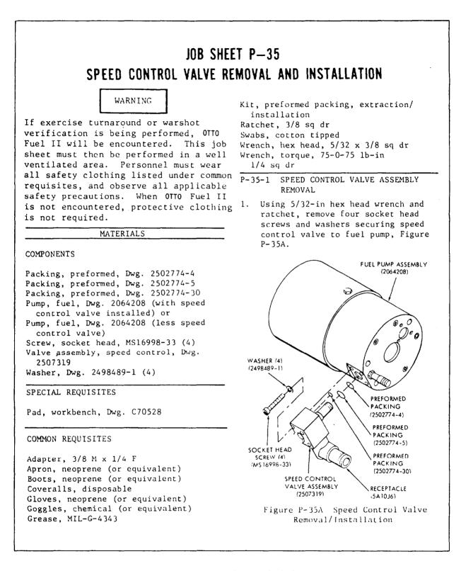
Figure 3-1.-First page of a typical job sheet.
