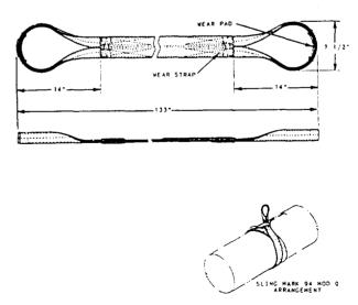
Figure 1-29.-Torpedo sling.
