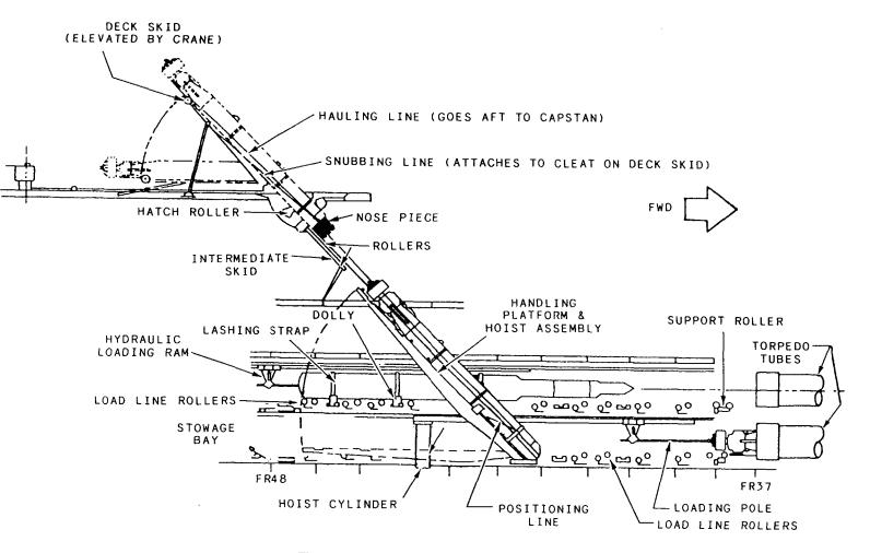
Figure 1-20.—SSN 637-class torpedo room.
