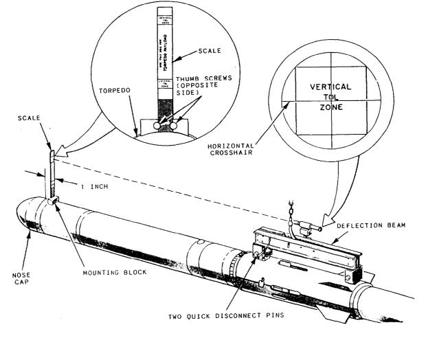
Figure 4-2.-Checking deflection of a rocket thrown torpedo.
