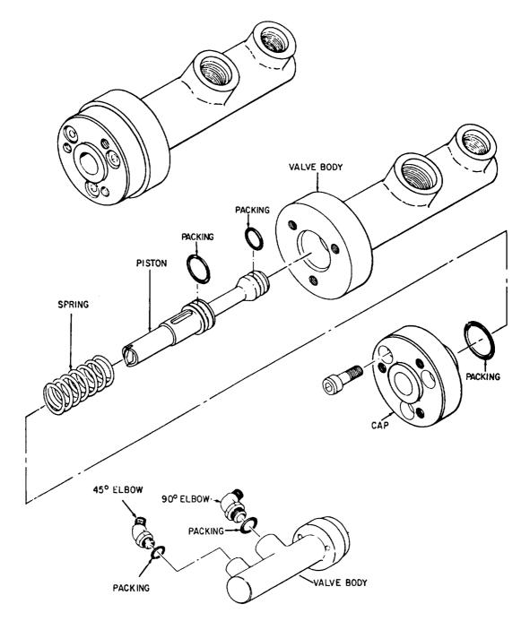
Figure 2-24.-Fuel interlock valve assembly.
