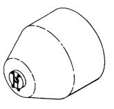
Figure 1-13.-Propeller guard for the Mk 46.
