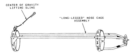
Figure 1-37.-Nose cage (Torpedo Mk 48, long-legged).
