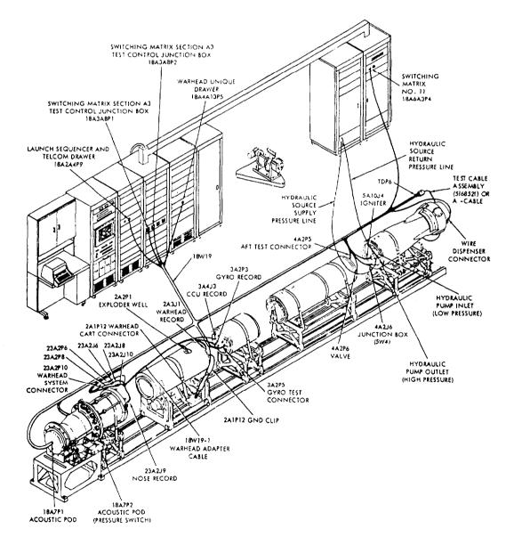
Figure 3-26.-Test connections for warshot torpedo system test.
