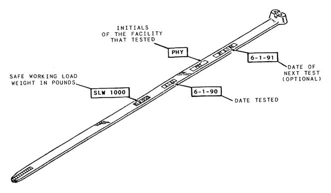
Figure 1-25.-Periodic load test record strap.
