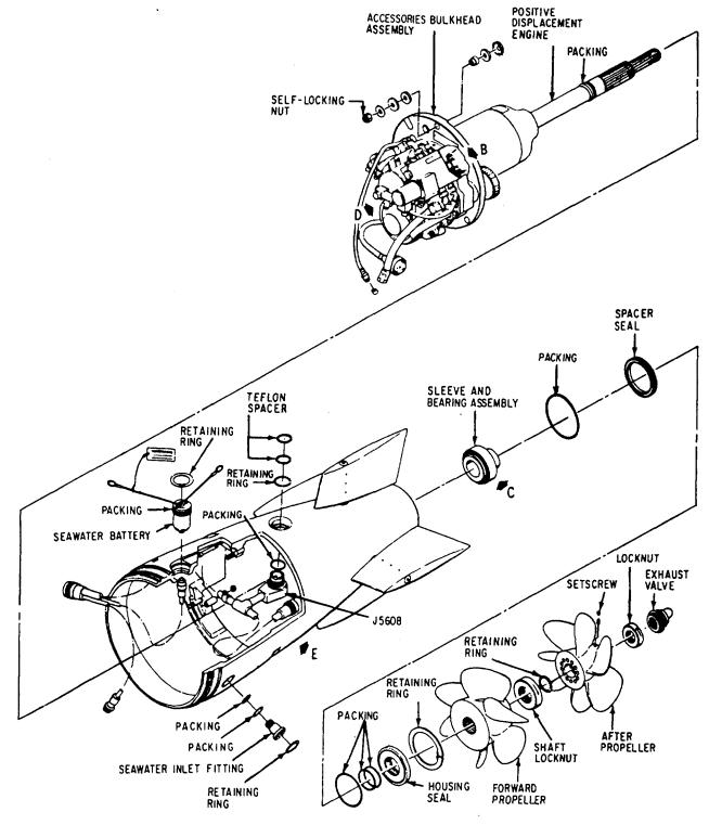
Figure 2-28.-Afterbody components.
