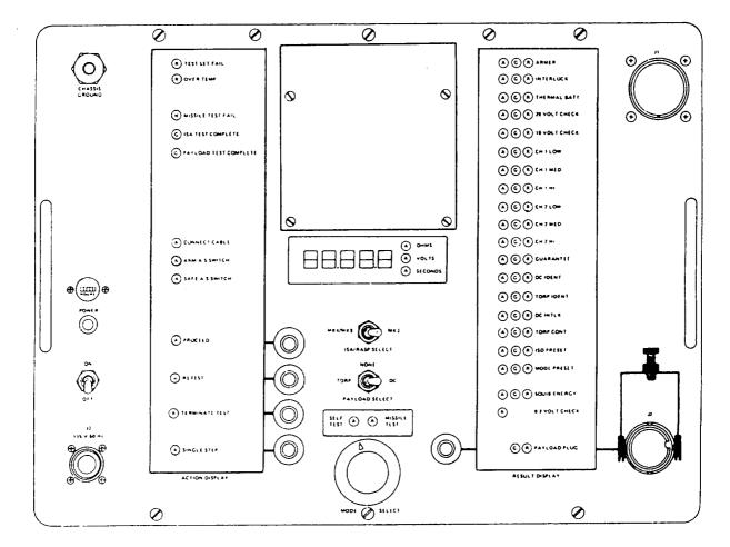
Figure 4-3.-Mk 620 Mod 0 test set.
