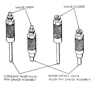
Figure 3-24.-Flush pin gauge assemblies.
