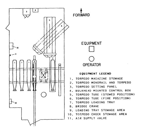
Figure 1-23.-Starboard torpedo room layout.
