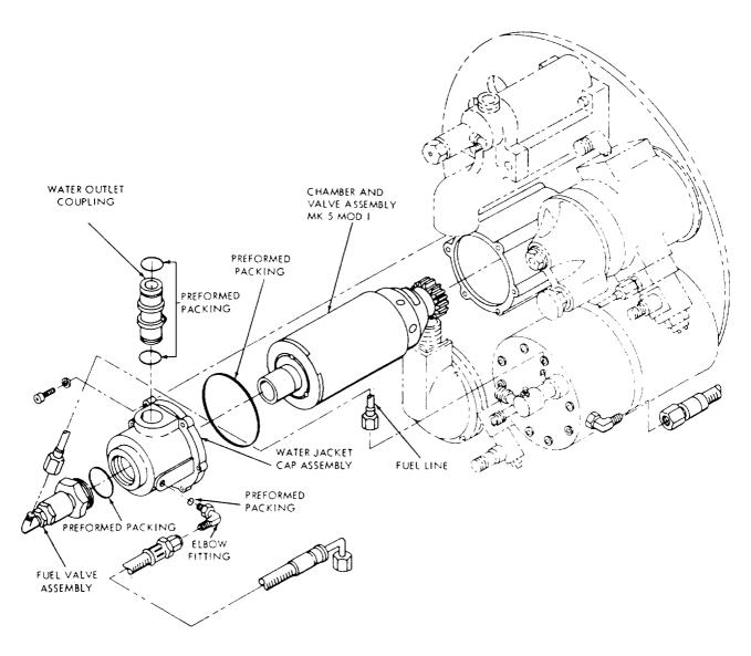
Figure 3-22.-Chamber and valve assembly installation.
