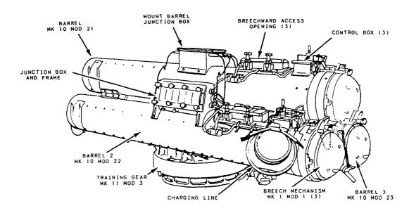
TORPEDO TUBE MK 32 MOD 14, STARBOARD CONFIGURATION, LEFT SIDE
