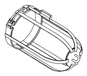
Figure 1-34.-Nose cage (Torpedo Mk 46).
