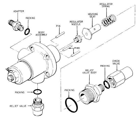
Figure 2-23.-Pressure regulator assembly (exploded view).
