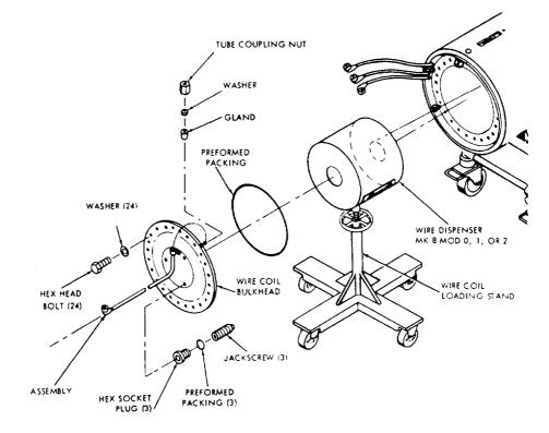
Figure 3-14.-Wire dispenser installation.
