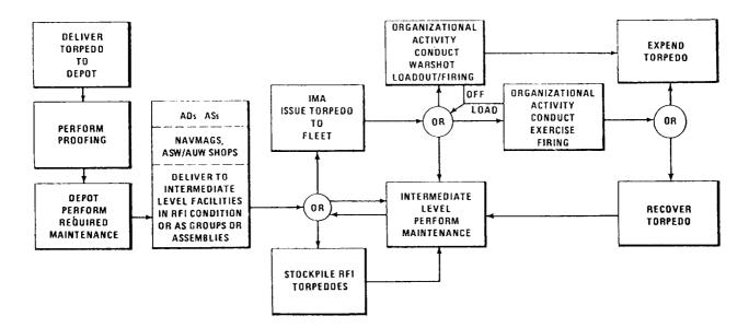
Figure 2-1.-Typical torpedo maintenance cycle.
