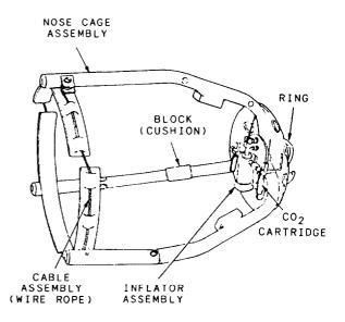
Figure 1-36.-Nose cage (Torpedo Mk 48 STD).
