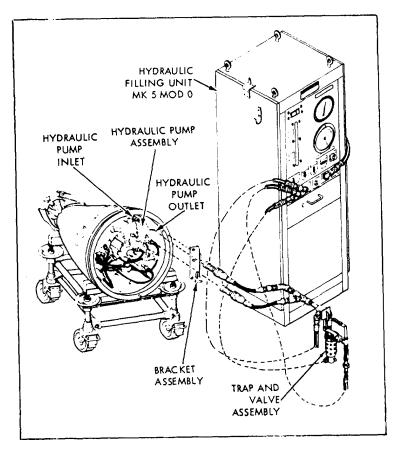
Figure 3-20.-Hydraulic system; drain, evacuate, and fill.
