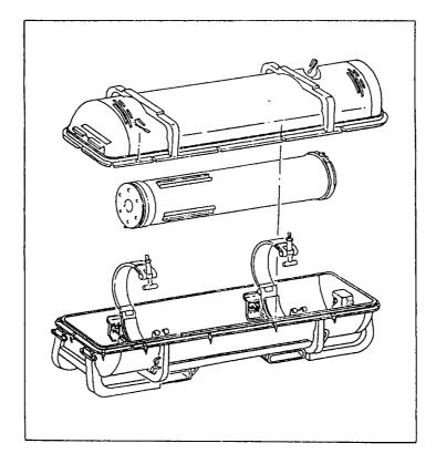
Figure 1-4.-Rocket motor Mk 37 container Mk 178.
