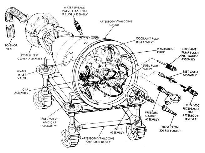
Figure 3-23.-Afterbody/tailcone accessory connections for operational test.
