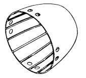
Figure 1-11.-Nose cover for the Mk 46 torpedo.
