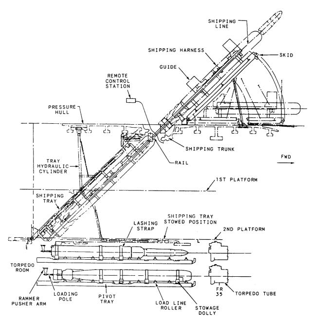
Figure 1-21.-SSN 688-class torpedo room.
