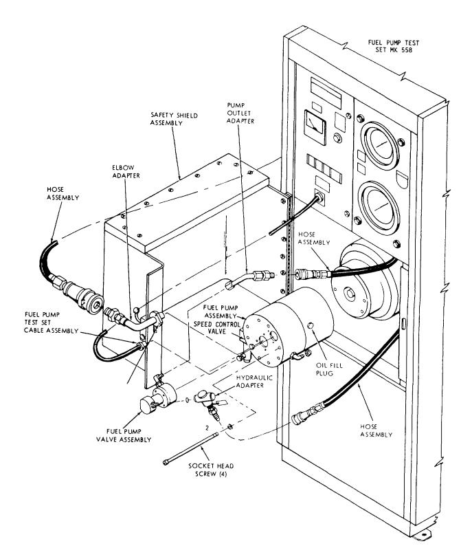
Figure 3-17.-Fuel pump/speed control valve test.
