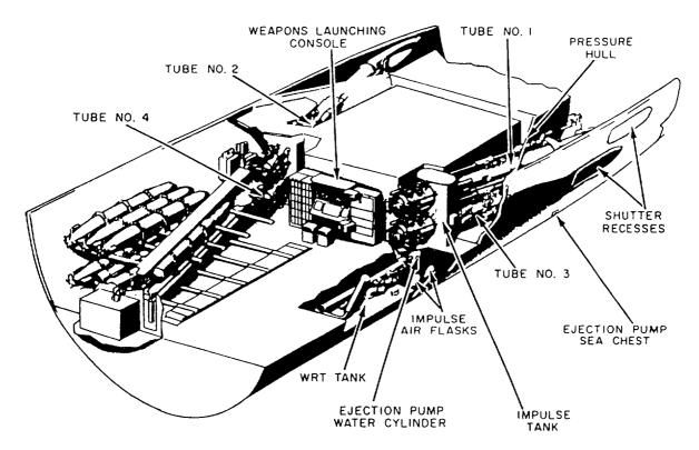
Figure 5-5.-Submarine Torpedo Tubes Mk 63.
