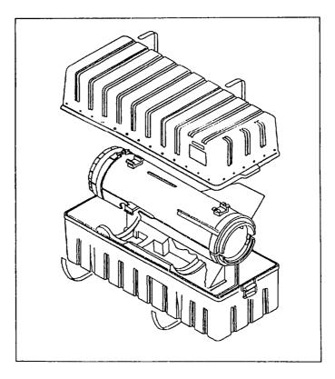
Figure 1-5.-Container for missile air frame.
