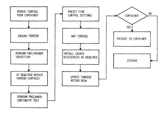
Figure 2-34.-Inspection flow diagram of fleet return torpedoes.
