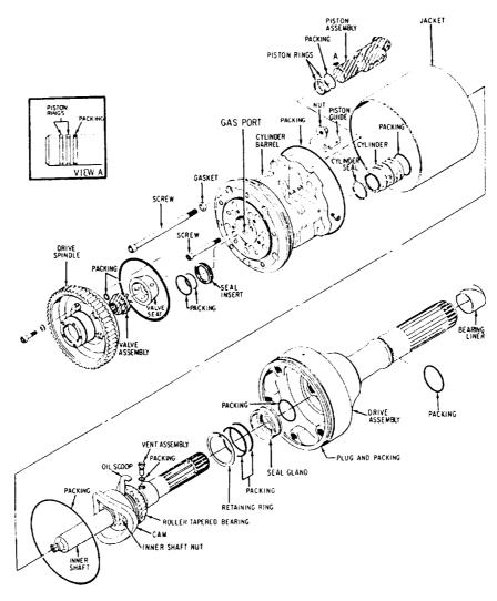
Figure 2-29.-Positive displacement engine.
