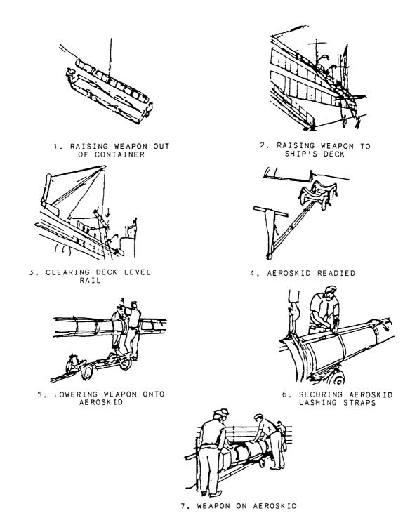
Figure 1-18.-Loading from dockside to the ship's deck.
