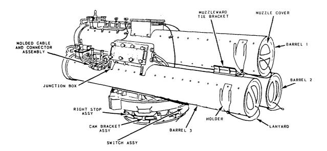
TORPEDO TUBE MK 32 MOD 14, PORT CONFIGURATION, RIGHT SIDE
