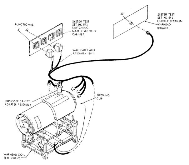
Figure 3-9.-Warhead group; FIR test setup.
