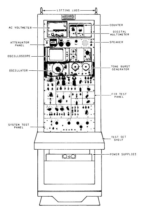
Figure 4-11.-Test Set Mk 572 Mod 0.
