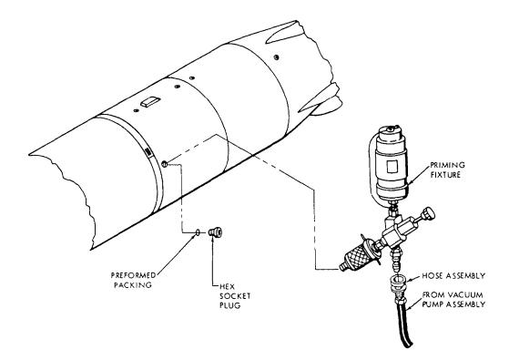
Figure 3-28.-Fuel pump priming.
