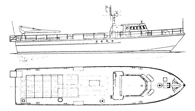
Figure 1-40.-A 85-foot torpedo recovery boat (TRB).
