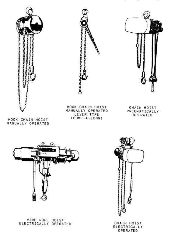
Figure 1-24.-Hoist and trolleys.
