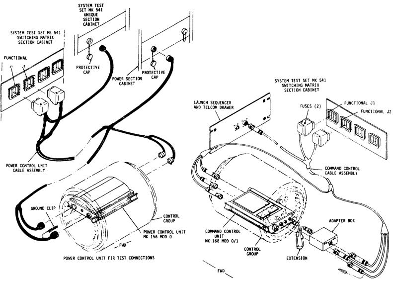
COMMAND CONTROL UNIT MK 168 MODE 0/1 FIR TEST CABLE CONNECTIONS
