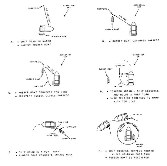
Figure 1-43.-Portable ramp recovery (diagram).
