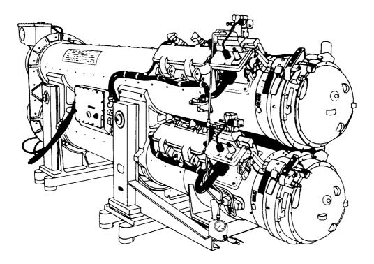
Figure 5-4.-Surface Vessel Torpedo Tube Mk 32 Mod 9.
