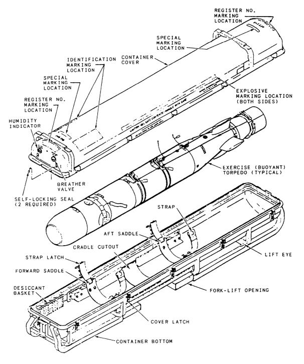
Figure 1-1.-Mk 46 torpedo container Mk 535 Mod 0.
