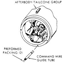
Figure 3-25.-Command wire guide tube installation in the afterbody/tailcone group.
