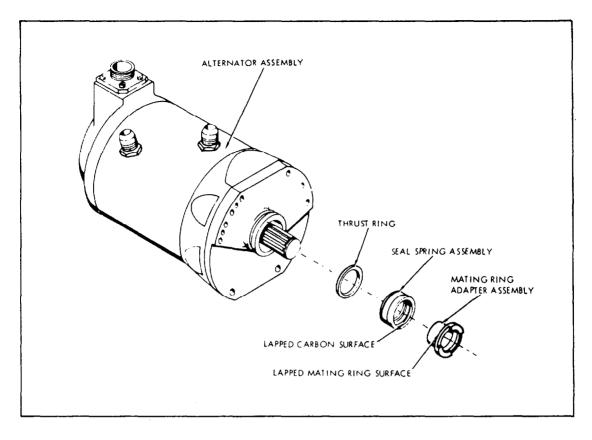
Figure 3-18.-Alternator sealol seal assembly; exploded view.
