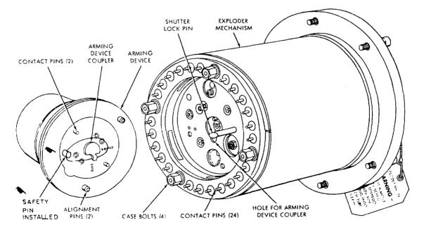
Figure 3-10.-Exploder mechanism and arming device.
