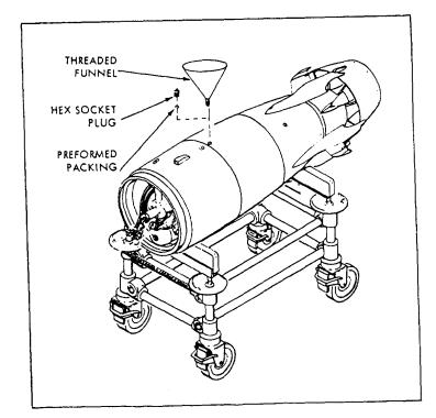
Figure 3-21.-Engine oil; fill.
