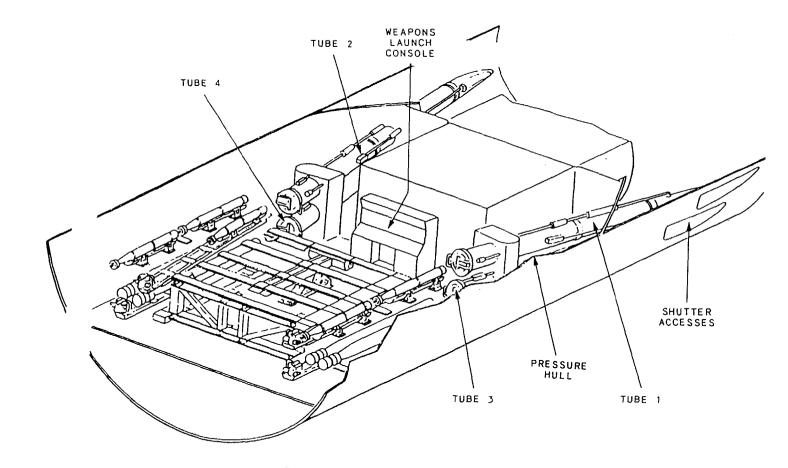
Figure 5-8.—Submarine Torpedo Tubes Mk 68.
