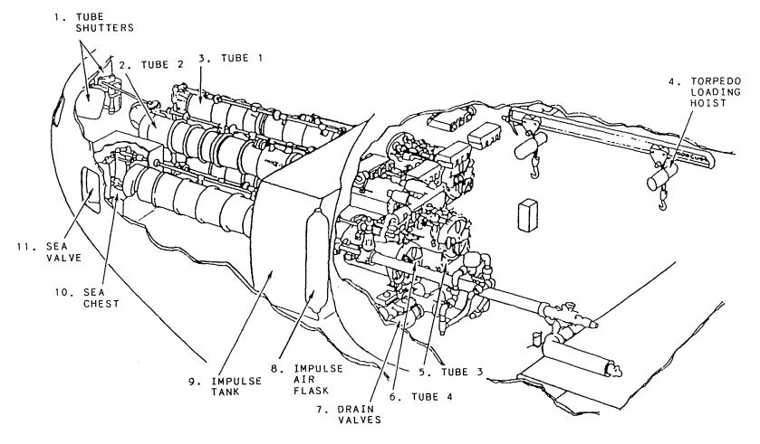
Figure 5-6.—Submarine Torpedo Tubes Mk 65.
