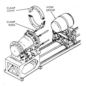
Figure 3-7.-Nose group in acoustic test stand.
