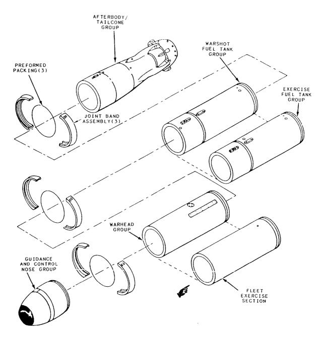
Figure 3-5.-Mk 48 ADCAP torpedo group configuration.
