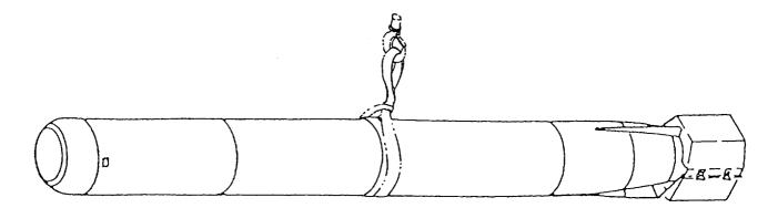
Figure 1-17.-Center of gravity.
