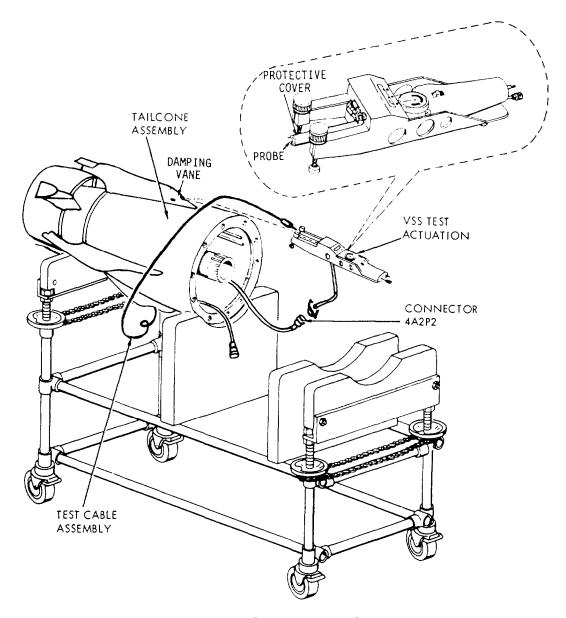
Figure 3-19.-Velocity sensor switch test.
