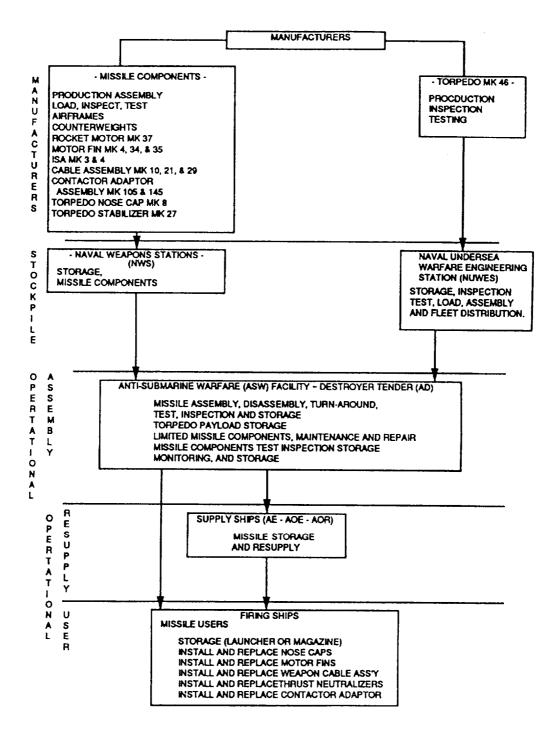
Figure 4-4.-Logistic flow chart for ASROC missile components/spares.
