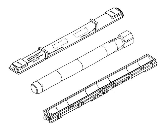
Figure 1-2.-Mk 48 torpedo shipping container Mk 481 Mod 1.
