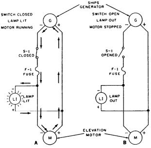
LI . INDICATES WHEN ELEVATION MOTOR IS RUNNING
