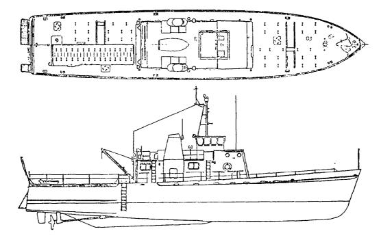
Figure 1-41.-A 102-foot torpedo weapons retriever (TWR).
