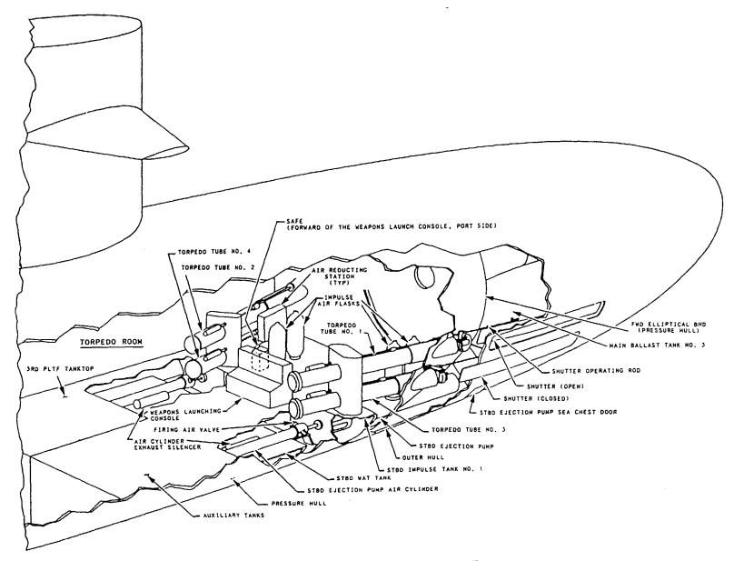
Figure 5-7.-Submarine Torpedo Tubes Mk 67.
