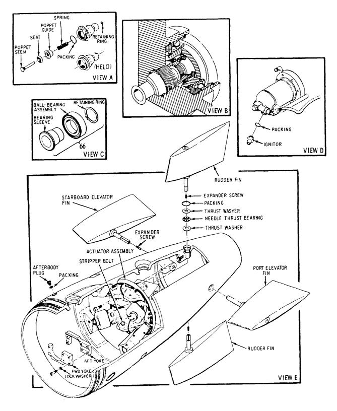
Figure 2-27.-Afterbody components.
