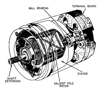
Figure 5-15.-Phantom view of a synchro.
