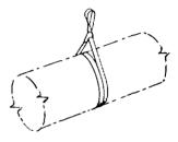
Figure 1-32.-Submarine simulator sling.
