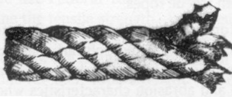
Three strand twisted or laid rope.
