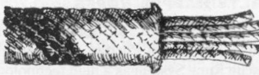
Dynamic, kernmantle rope used for rock climbing.
