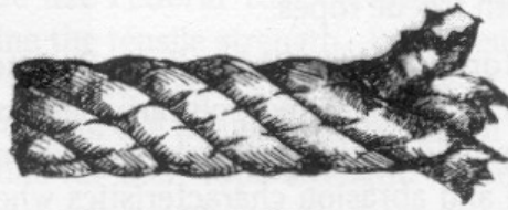
Three strand twisted or laid rope.
