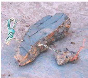
Remote control receiver hidden in plaster.
