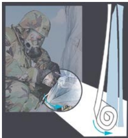
Secure barrier material. Roll excess material beneath asset, away from contaminants.
